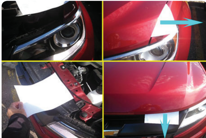
Check for proper contact of the outer and middle bumpers to the hood.
