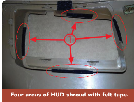
Felt tape applied to the full perimeter of the HUD shroud.
