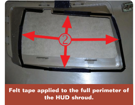
Four areas of HUD shroud with felt tape.
