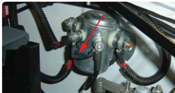
Insulate the diode with heat shrink tubing before installation.
