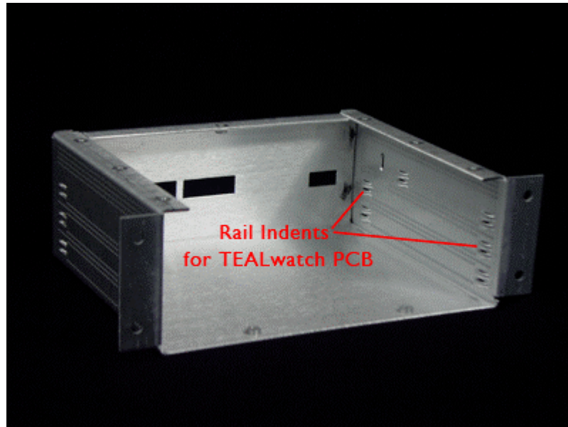
Figure 6.3.6 – Use center rail indents to re-install main PCB. Connectors should line up with holes in front and back of enclosure.
