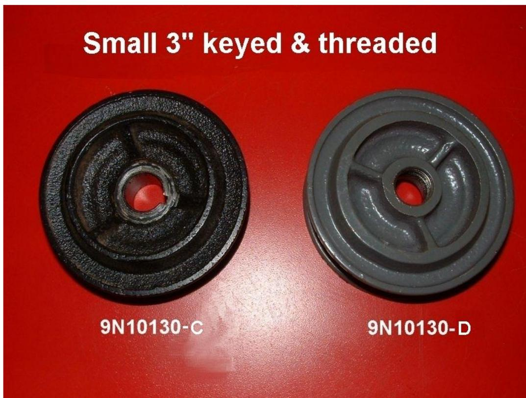
**FIG. 10 –The smaller 9N-10130-C and 9N-10130-D Pulleys. Designed with a smaller Major OD at 3-3/16" and therefore a smaller Over-The Roll\* dimension. Note the 'C' is keyed and replaced the 'A' pulley and the 'D' is threaded which replaced the 'B' pulley.**
