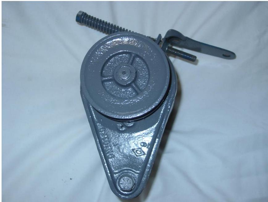
**FIG. 15 –The 2N-10000 Generator & Tensioning Bracket Assembly. Front view.**
