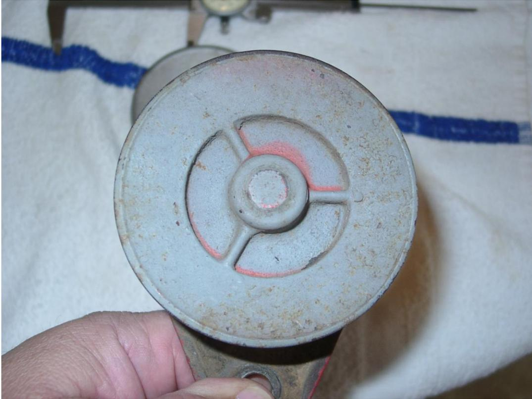
**FIG. 9 -9N-10130-B Pulley. Threaded with .59-20 thread –not an industry standard nominal size. It is a Metric/Inch hybrid but system was used on cars and trucks as well, not just the tractors.**
