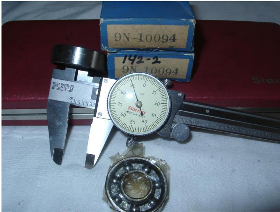
**Fig. 19 – Generator bearing 9N-10094 as shown with the ID measuring .59" which is equivalent to 15mm. Bearings were in metric, thus the armature shafts and their fasteners were as well.**
