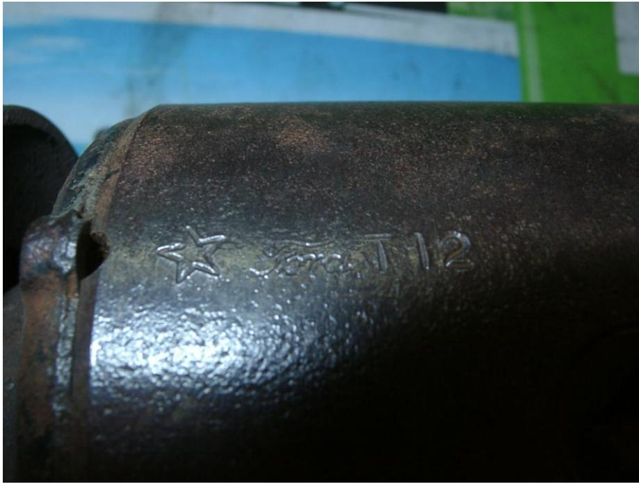
**FIG. 4 –The Date Code stamp on a 9N-10000-A Generator. T12 denotes December 1939 which identifies when the unit was built.**
