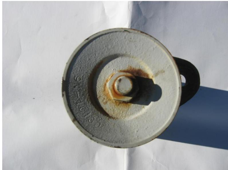
**FIG. 5 -The 9N-10130-A Pulley. The cast iron unit featured a 3-11/16" major Diameter, 3-1/2" Effective Diameter; .59" [15mm] bored ID with a 1/8" keyway broached thru, and part number cast in recessed characters. The armature end was threaded at .59-20 and fastened with a lockwasher and special hex nut.**
