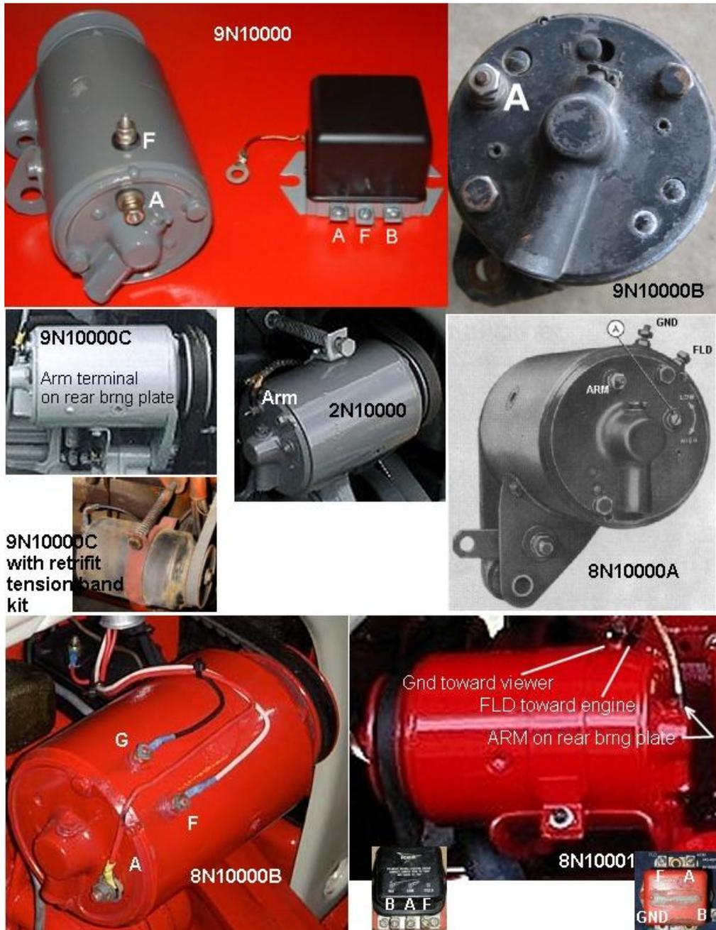
**FIG. 15–Visual Aid –all the 9N and 2N generators with the 8N models shown.**
