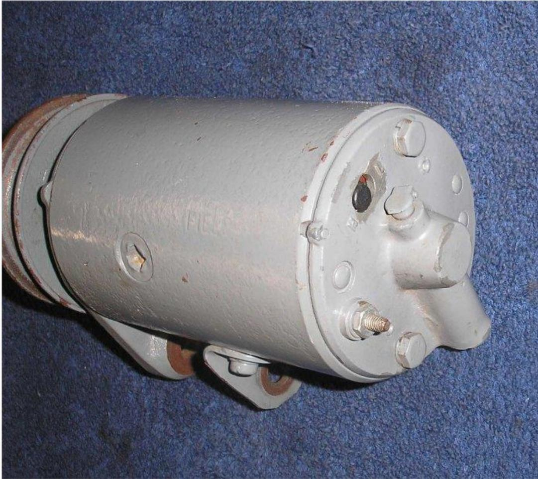
**FIG. 8 –The 9N-10000-B Generator, a 3-brush, 1-wire design. Rated current output was 7 amps at 7.5 volts. Note black HI-LO 3rd brush adjustment button.**
