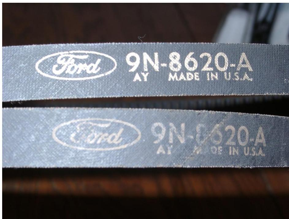
**FIG. 16 –NOS Ford fan belts 9N-8620-A. This is the correct belt to use with the early small 'A' and 'B' generators.**
