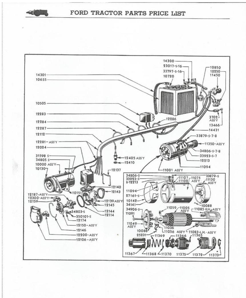
**FIG. 1 –March 15, 1940 Master Parts Catalog, page 34, shows detailed drawing of electrical wiring. Note the square-case voltage regulator, 9N-10505.**
