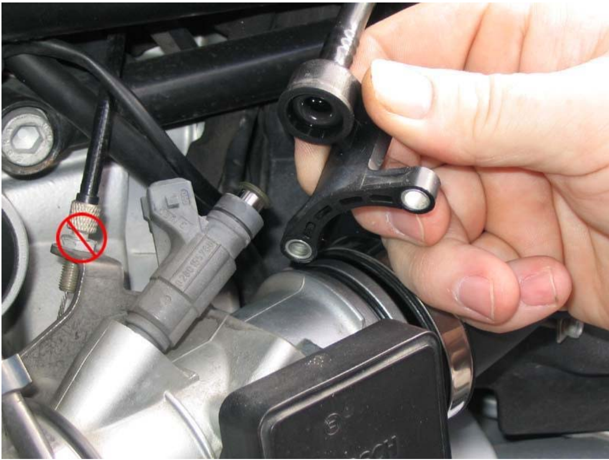
Look at that, the o-ring stayed with the fuel line end cup.
