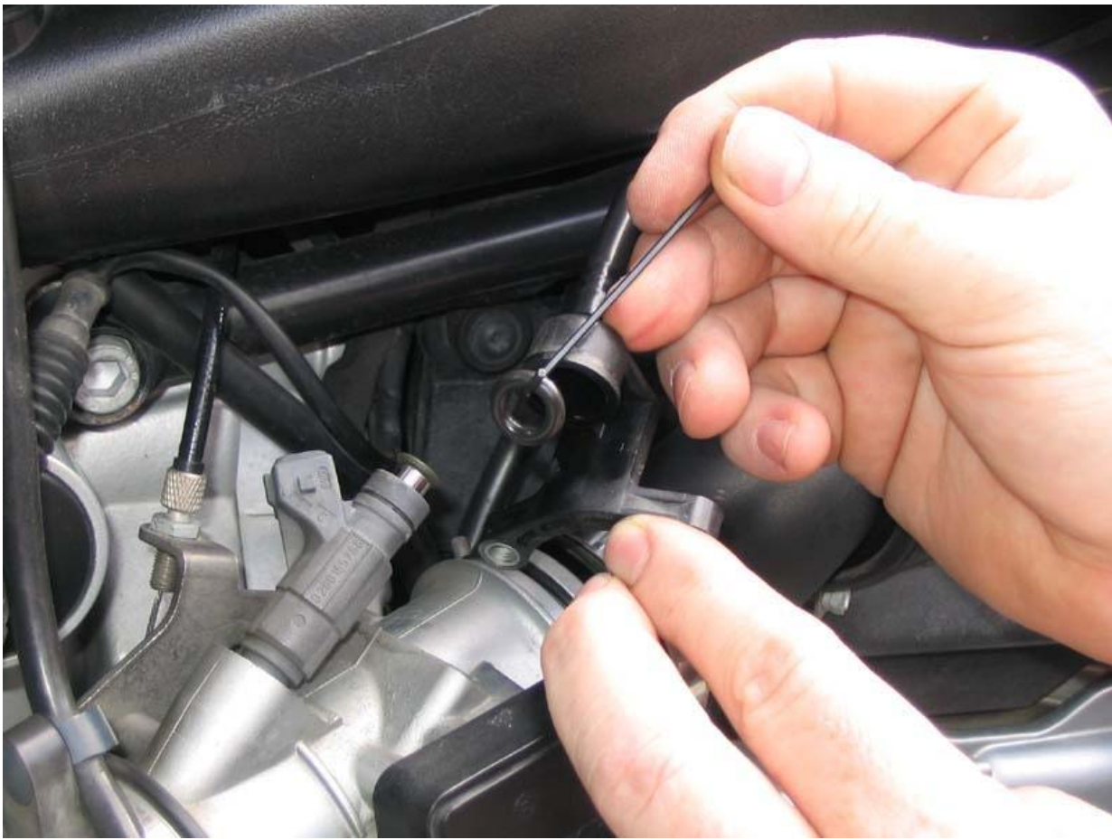
Pull out the fuel injector.
