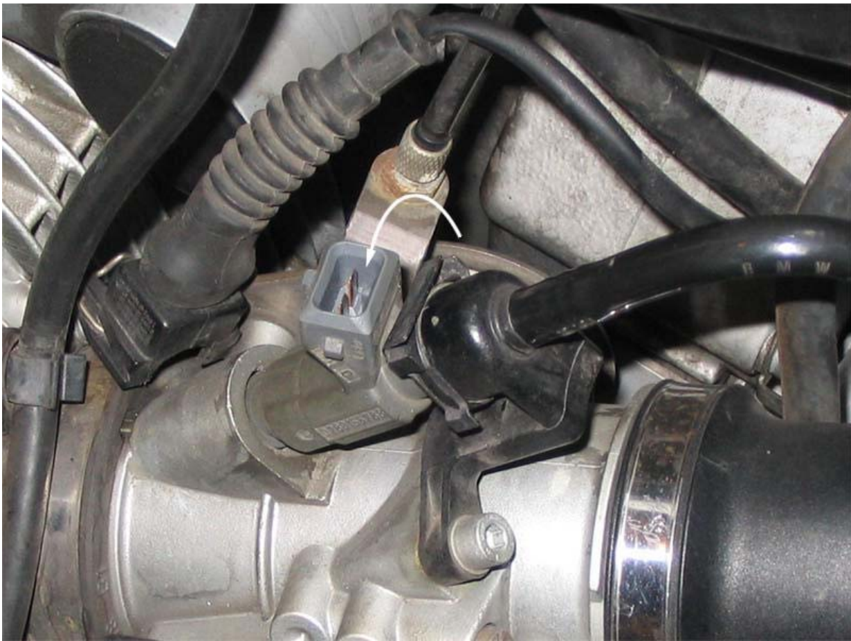
Plug in the electrical connector. When oriented correctly, the electrical connector blocks the injector retaining clip.
