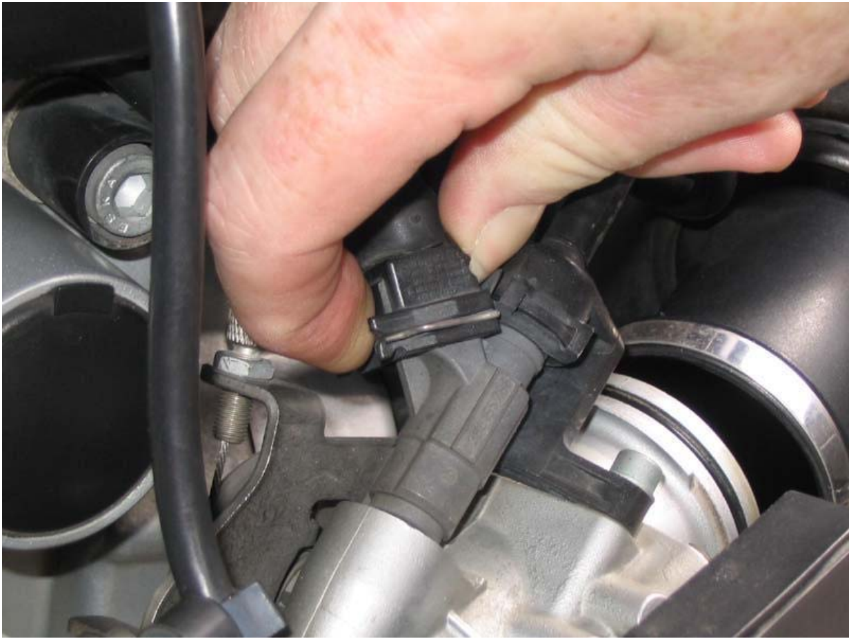
Remove the fuel line retainer spring clip.
