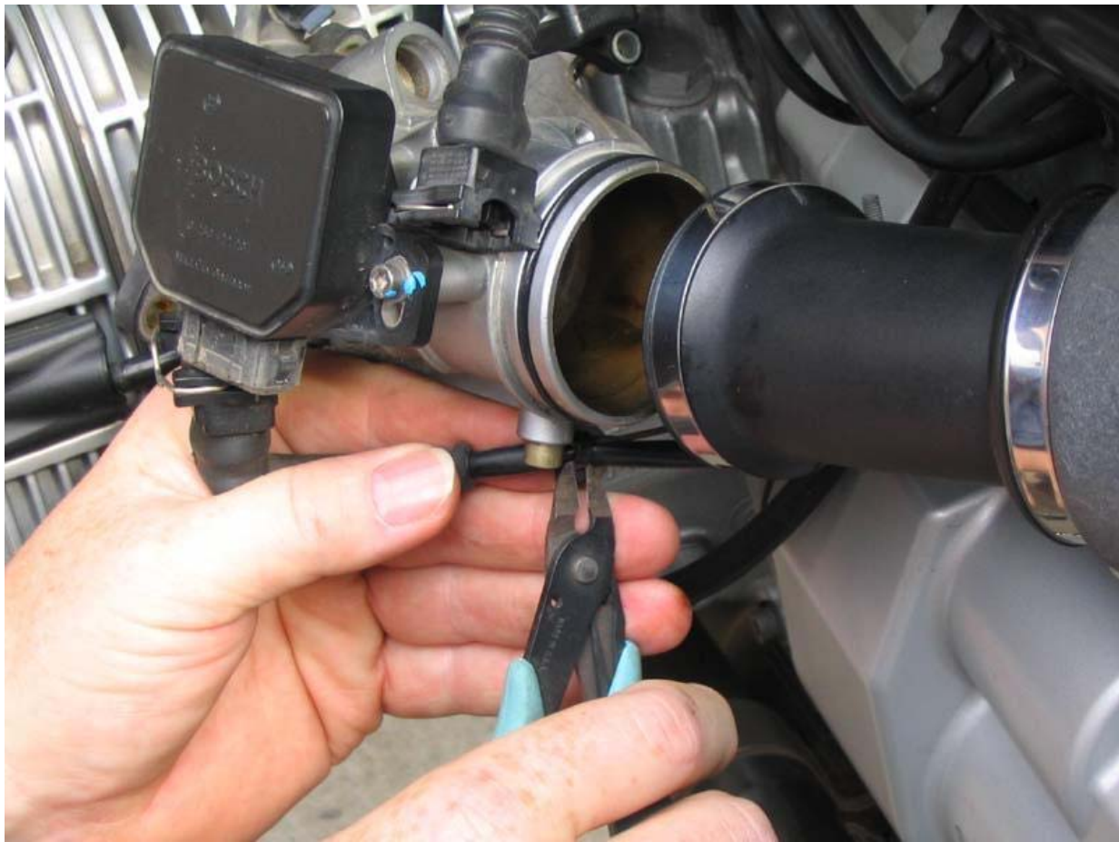
Remove the throttle body ground lead.
