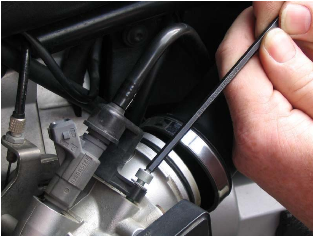
Pop off the injector fuel line.
