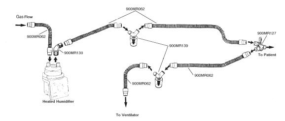
Parts required for a suggested circuit configurations are as follows:
