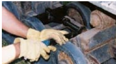
Picture 51 – Adjusting track length
