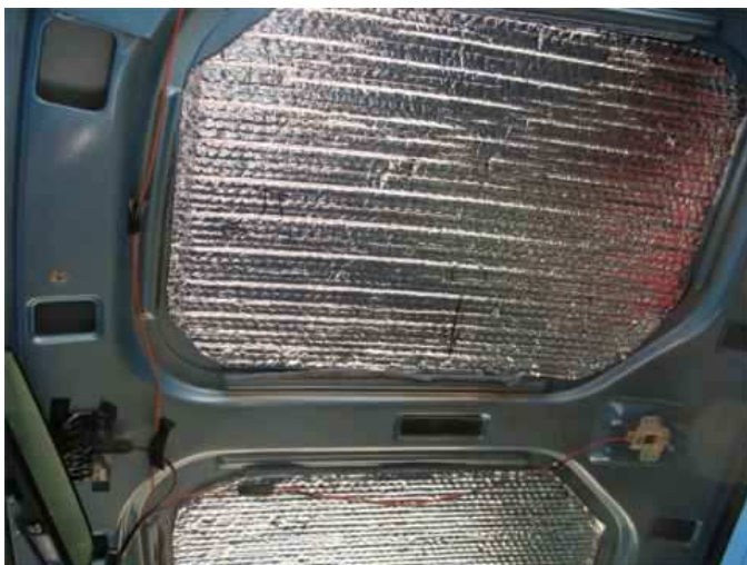
New headliner insulation
