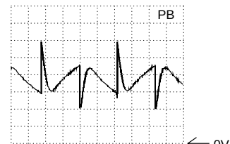
DC, 1V/Div, 500μs/Div IC7095-(14)
