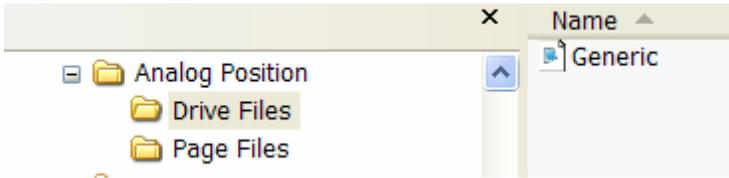
The Drive File directory contains a list of drive files for this application. The Drive file contains the upload and down load parameter values as well as parameter names, Modbus addresses, scaling, default values. The parameter values in the Drive File is the data actually downloaded / uploaded from the drive. Drive file is named Generic in above example.
