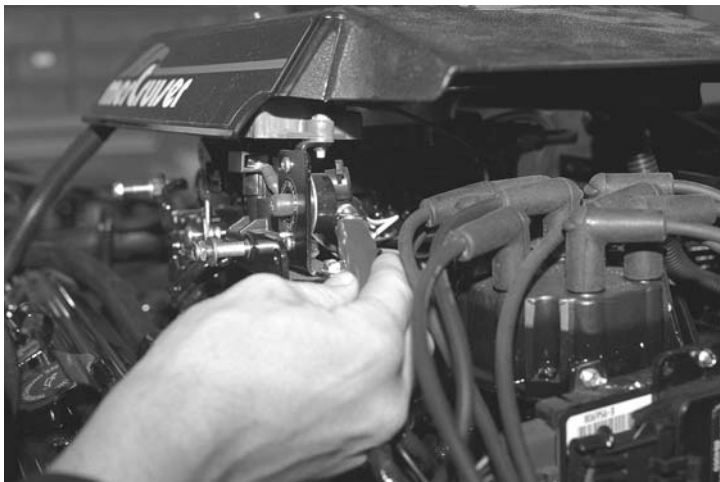
Figure 12 Circuit Breaker Terminal
