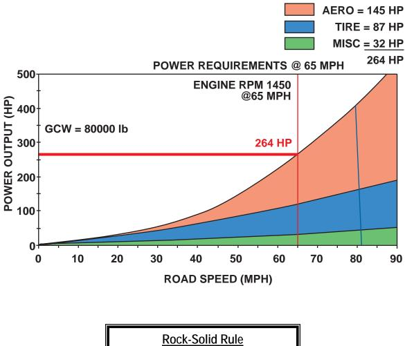
Tires make biggest difference in MPG below 50 mph; aerodynamics is the most important factor over 50 mph.
