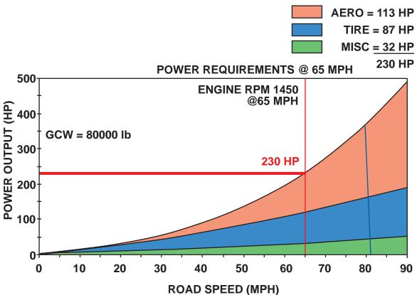
Notice that these aerodynamic treatments are more effective at higher speeds as represented by the increased vertical depth of the red graph above. Also notice that the power required to overcome things like tire rolling resistance are not affected by the aerodynamic aids.
