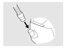
**2** Connect the other end of the patient tube to the mask and the ventilation valve, if applicable.
