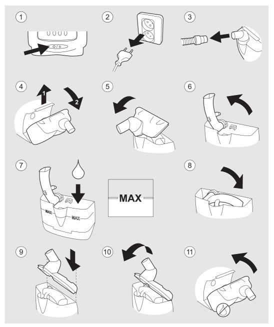
Add distilled water or boiled, chilled tap water to the humidifier until it reaches the marking "Max" on the humidifier. A full humidifier contains approximately 400 ml. Do not overfill the humidifier.
