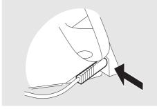
**2** Turn on the iSleep 20+ by pressing the Start/Stop button on the front panel for 2 seconds.
