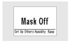
If the patient removes the mask, the iSleep 20+ will minimise the pressure to approximately 1 cmH<sub>2</sub>O (the pressure level depends on the mask type). When the patient has put on the mask again and taken a few breaths, the iSleep 20+ will go back to the pressure delivered before the patient removed the mask.
