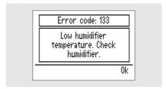
133: Low humidifier temperature. Check that the humidifier is connected correctly (this error is shown after the treatment session). If the error remains, contact your care provider.
