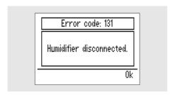
131: The HA 01 humidifier has been disconnected when the iSleep 20+ was running. Always turn of the iSleep 20+ before disconnecting the HA 01 humidifier.
