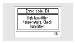
134: High humidifier temperature. Turn off the iSleep 20+. Disconnect the humidifier and reconnect it. If the error remains, contact your care pro-
