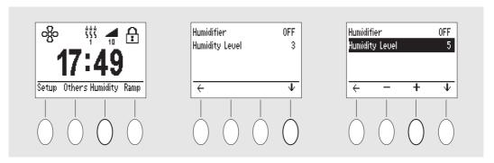
Use the 4 buttons under the display to navigate in the menu. Depending on the location in the menu, the buttons have different function. The following icons are used:
