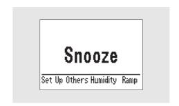
In order to start the treatment again, start to breath in the mask or press the Start/Stop button shortly. The iSleep 20+ will then increase the pressure to the set level during up to 10 seconds.
