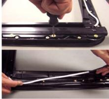
Remove the mechanism guide and drive cable center plate T-25 torx screws.
