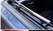
Click the front hook of the locking slider on the mechanism.
