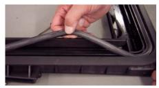
Remove the seal section from the mainframe.
