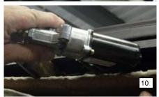
Remove the motor assembly.
