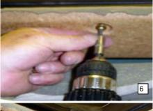
Remove the T-25 screws retaining the bezel to the mainframe. (450 HS only)
