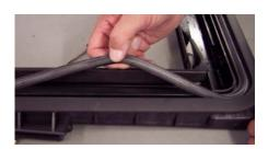
Insert the new seal, starting in the four corners. equally dividing the seal.
