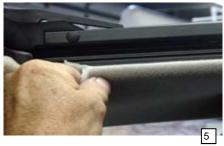
Carefully peel back the headliner material to gain access to the attachment screws. (450 HS only)
