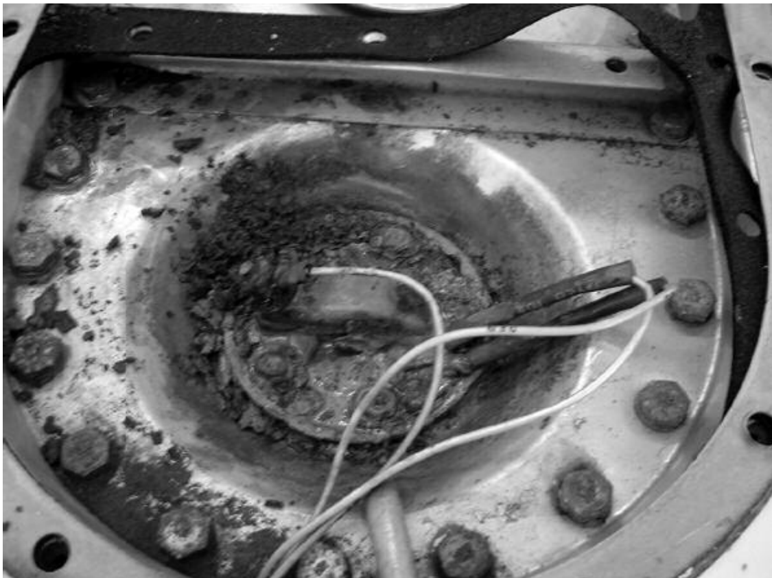
This main tank transmitter didn't survive due to the extensive corrosion.
