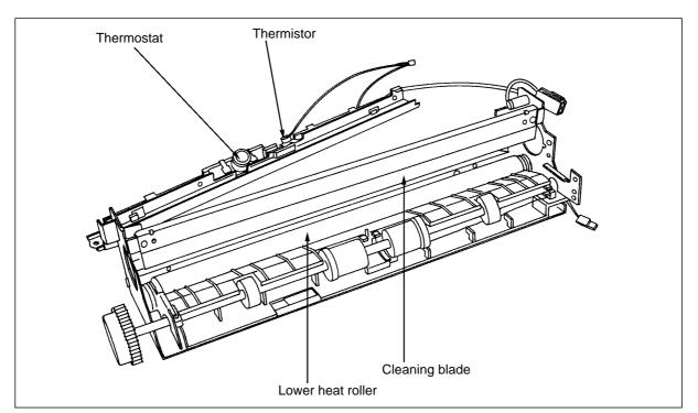
View with the upper heat roller removed
