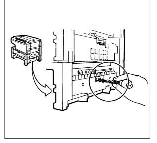
(3) Plug the connector of the paper guide (1) into the connector J36 from the feed side of the MY-1004.
