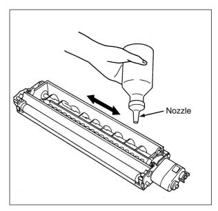
(3) After pouring in the developer material, rotate the gear in the direction of the arrow as shown to deliver the developer material onto the magnetic roller.
