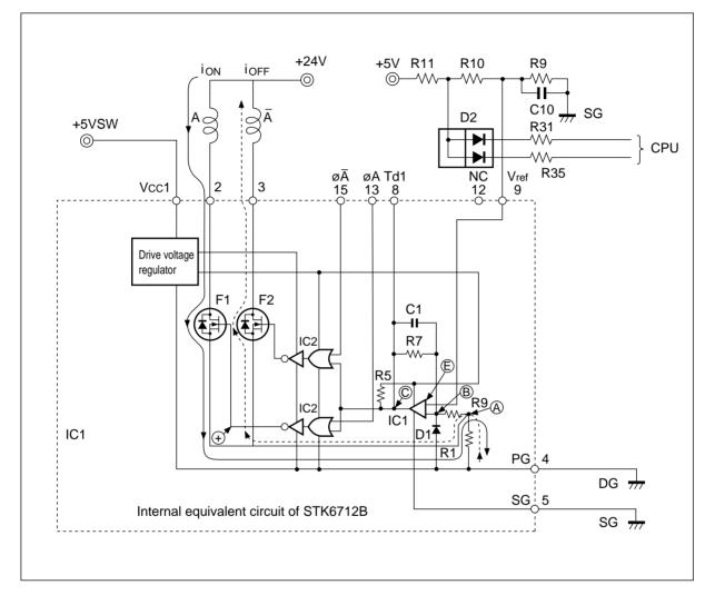
The circuit composition in the IC consists of each phase excitation switching section (IC2), a driver (F1, F2), a comparator (IC1) and an electric current detection resistance (R11). The circuit operation in the case of excitation of phase A is described below:
