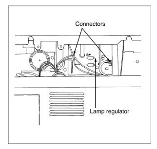
(8) Remove the exposure lamp and power supply connector.
