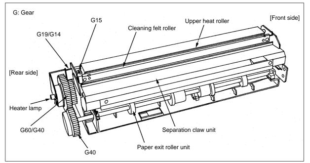
View with the fuser guard removed
