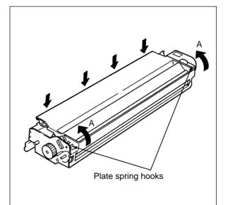
(5) Pay special attention to the overlapping of the side shields (front and rear) and the rubber seal when installing the top cover; the rubber seal should be over the side seals.
