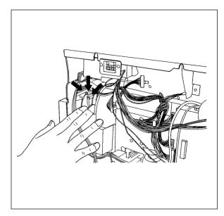
(11) Disconnect the connector for the process unit.
