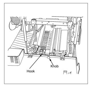
(4) Remove the transport guide (1 screw and 1 blue connector at the rear).
