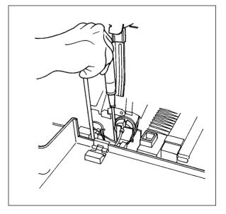
(7) Remove the lamp regulator (two connectors).
