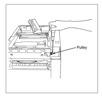
(8) Loosen the screw for the wire take-up pulley located inside the frame
