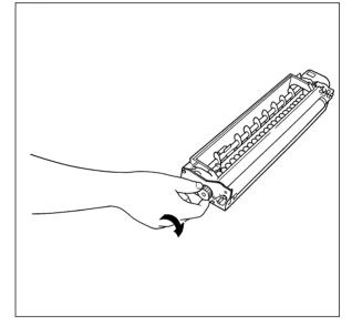
(4) Reinstall the top cover; after inserting the hooks(4 places) firmly, fix the plate spring hooks by rotating in the direction of arrow A securely.
