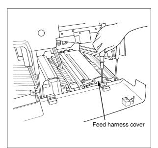
(3) After removing one screw and disconnecting one connector, pull the unit out to the front and lift it out.
