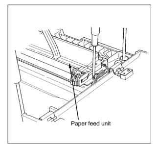
(6) Remove the lower drive unit bracket (1 screw) and separate the drive unit from the bracket (2 screws).
