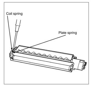
(3) Remove the adjuster plate (1 screw).(Before removing it, memorize its original position.)
