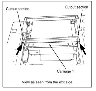
(4) Slanting the whole carriage 1 unit, take it out upwards.
