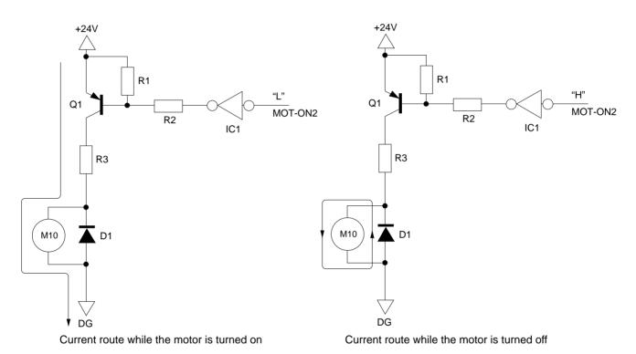
\*1: The MOT-ON2 signal is to cause the motor (PFU-MOT) M10 to rotate and is supplied by the copier. When this signal becomes "L", the motor starts rotating.
