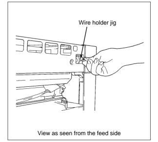
(4) After having loosened the wire tension adjustment screw, disengage the hook on the feed side
