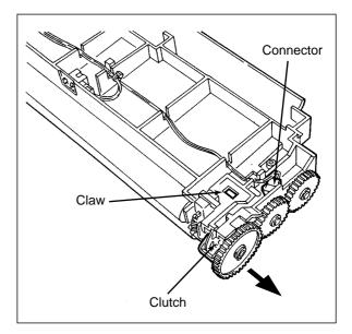
(6) Removing one setscrew allows the clutch and the aligning roller (lower) to be disassembled, respectively. Also, the aligning roller (upper) can be removed.
