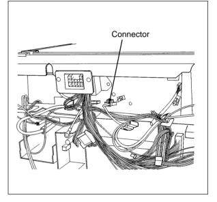
(9) Disconnect the connector for the auto exposure, lens switch and mirror motor.
