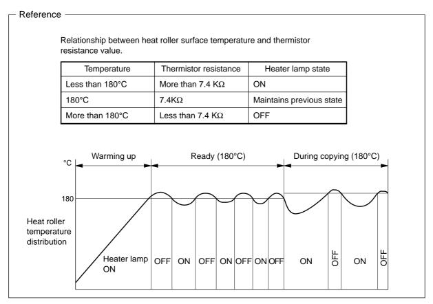
(2) Thermistor disconnection detection
