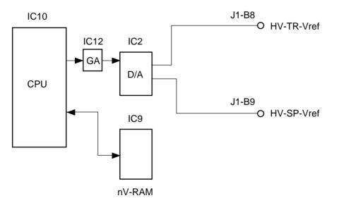
Transfer/separation control circuit diagram
