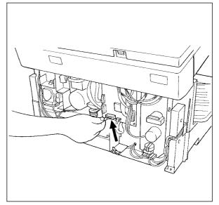
• After pulling out the whole unit to the front side, remove one claw and raising the switch, disconnect the connector.
