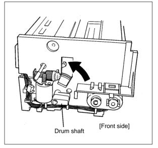
When removing the drum, place your hands on the sides of the drum, as shown in the figure on the right and take it out carefully.
