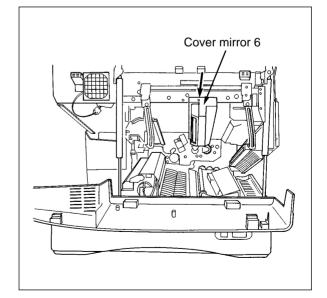
(3) Remove the transfer/separation charger (Refer to 9.3.6).
