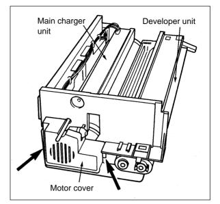
• Unlock the drum shaft lock (by rotating it in the direction of the arrow) and then pull the shaft out from the front.
