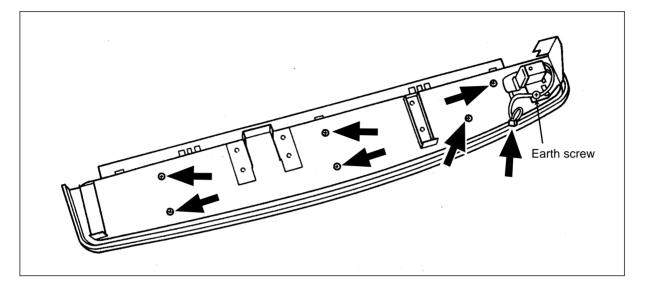
(3) When you remove nine (9) screws, the control-panel PC board can be taken out along with the harness. They can be separated if you disconnect two connectors.
