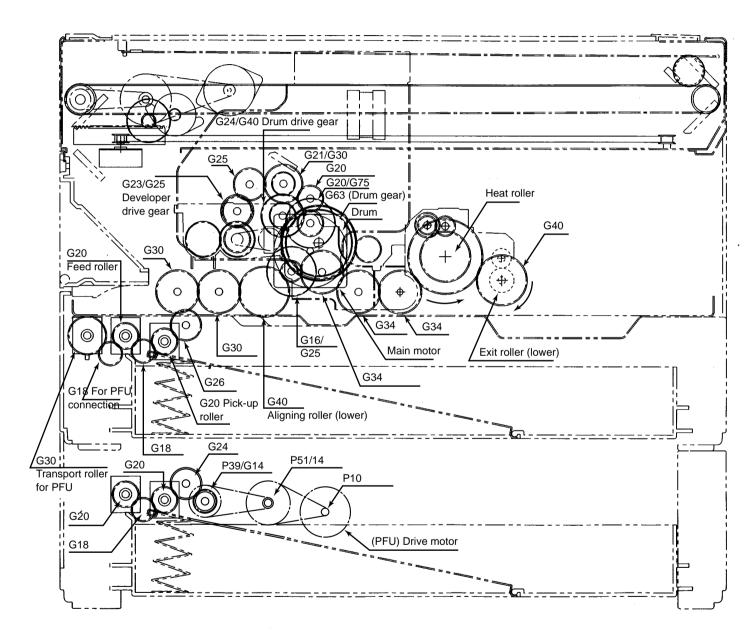
All parts except the main motor are located inside the frames.
