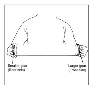
2. After inserting the drum shaft, apply patting powder on the entire surface of the drum and rotate the drum toward you.
