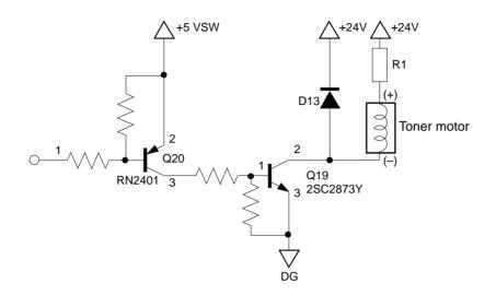
The (+) and (-) terminals of the motor winding is connected to +24V and pin 2 of Q19, respectively.
