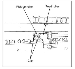
Note: The separation, pick-up and feed rollers are the same parts as used in the copier. Caution: During disassembly or reassembly, be careful not to lose the spring.
