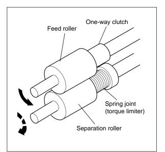
For example, when only one sheet of paper (1) is sent to the separation area, since the feed roller's transporting force is stronger, the separation roller is forced to rotate in the direction of the arrow ( $\cancel{}$ ), causing the sheet to be sent toward the aligning roller.
