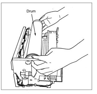
Notes: 1. When setting the drum in the process unit, its smaller drive gear should be on the rear side.
