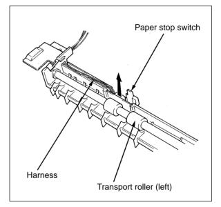
When reinstalling the transport paper guide, make sure that the plate spring is in contact with the shaft of the transport roller (right) securely.
