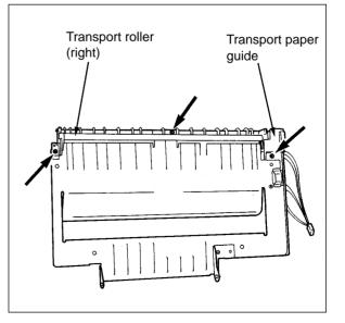
(3) While bending the transport guide in the direction of the arrow, remove the bushings from the frame
