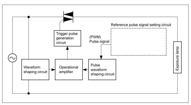
The voltage applied across the lamp is kept consistent.
