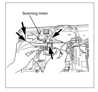
(7) Remove the pulley on the rear side (1 screw).
