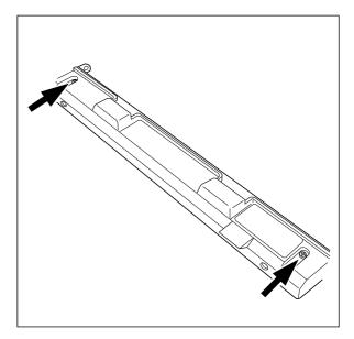
(4) Remove the bracket from the separation claw unit (4 screws).
