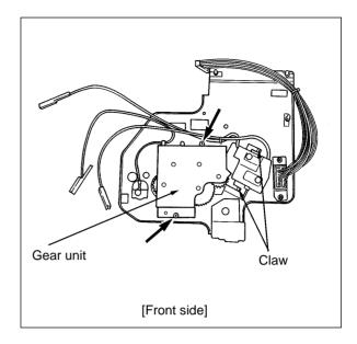
(3) After removing the two claws on the front side, slide out the main charger terminal to the right.
