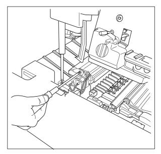
(3) Remove the upper cover of the separation claw unit (2 screws).
