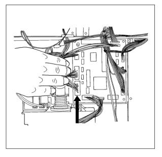
(12) Remove the drive unit from the rear inside of the machine (3 screws).
