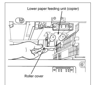
(3) Remove one screw from the lower paper feeding unit.
