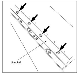
(5) Remove the lower cover (4 screws). (1 unit : screws 2×2) Take off the six claws from the claw holder.
