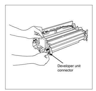
(3) Lifting the levers, take out the developer unit.
