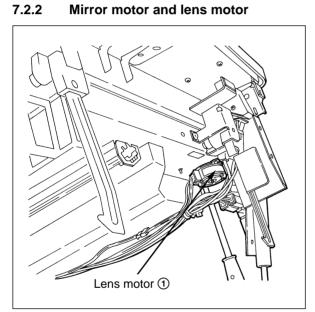
View with the process unit and the stay removed and the upper unit raised
