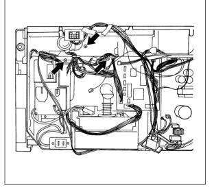
(13) Removing two screws, take out the bracket and the gear can be replaced.
