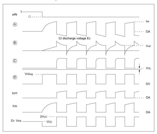
Shown below is the waveform timing chart of each section:
