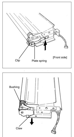
(3) While pushing down the claw, pull out the bushing toward the front.
