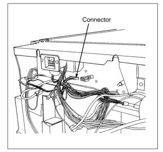
(10) Pull out the three connectors for the main charger and the bias wire from the high-volt-age transformer.
