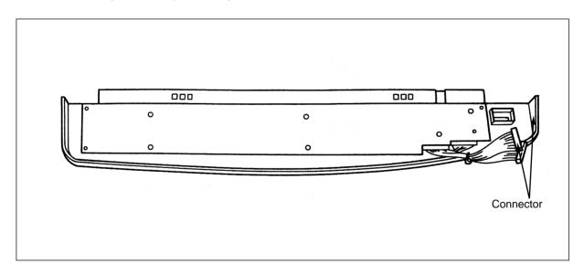
Note: Be careful not to allow the ground wire of the shield to be cut.
