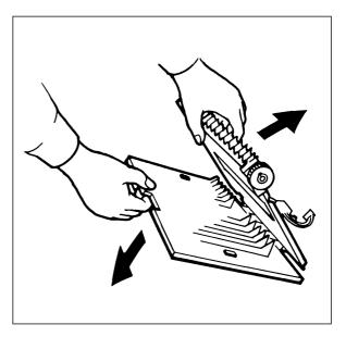
(2) Insert the separation roller pressure spring
