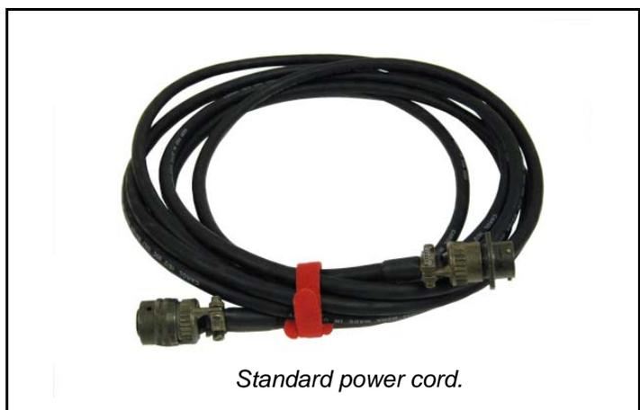
A bench test power cord is also provided. One end of the cord is provided with a receptacle to connect to the pigtail cord on the main control panel. The other end of the cord is fitted with 1/4" ring terminals for attachment to an external power supply/battery for bench test purposes.
