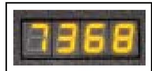
The lifetime count of spheres is displayed on the segment LED by pushing the “RESET” toggle switch *momentarily*. The lifetime count equals the number displayed multiplied by 1000. These counts are maintained in memory even when the unit is powered down.
