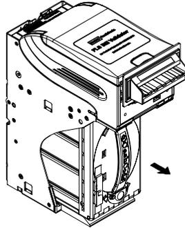
To replace the Cassette, close the Cassette cover, insert the Cassette into the FrontLoad frame.
