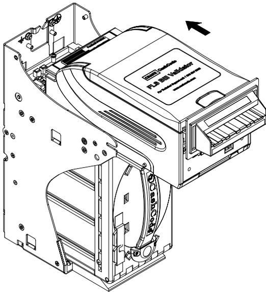
5.1.5 Turn Power ON and wait until the download process is completed. During the download, a red-green status light will blink. Once the download is completed, the diagnostic light will turn green. If the light stay red, this means there is no communication between the FrontLoad Bill Validator and the host controller
