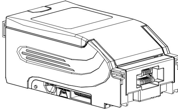
**2.4. Housing:** The Housing is made of rigid metal structure, which allows you to mount from left / right or back side.
