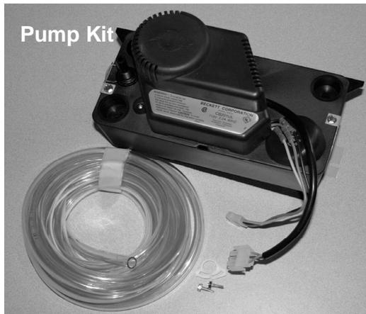
The condensate pump provides for the automatic removal of condensate water during the cooling process. The pump is capable of pumping against a 20 foot head, allowing for the routing of the drain line above the drop-ceiling to a nearby drain. The pump is controlled by an internal float-switch which turns the pump on and off automatically. The pump is also equipped with a condensate over-flow safety switch, that will shut down the ARCTICAIRE compressor when the pump is not working prop-
