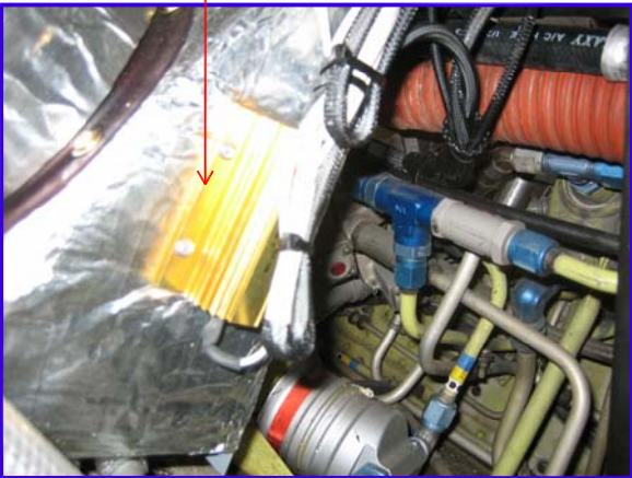
A/C SPEED CONTROL RESISTOR PN: 050024-2
