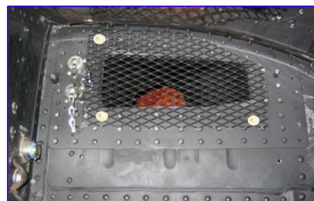
RETURN AIR SCREEN PN: 080036-P ABOVE AND BEHIND CO-PILOTS HEAD.
