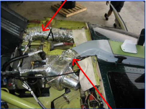
COVER DUCT WITH FOAM AND ALUMINUM TAPE.
