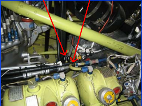
#10 HOSE ASS'Y P/N: 5700059-O-P HIGH PRESSURE SWITCH P/N: 090004
