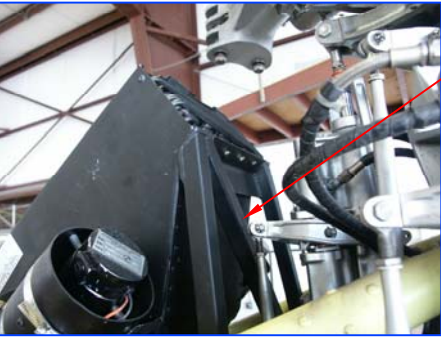
COND. SUPPORT MUST CLEAR ALL CONTROLS COND. SUPPORT MUST CLEAR TRANSMISSION SUPPORTS
