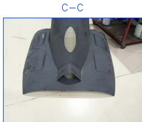
CONDENSER AIR INTAKE IN COWLING, EXISTING
