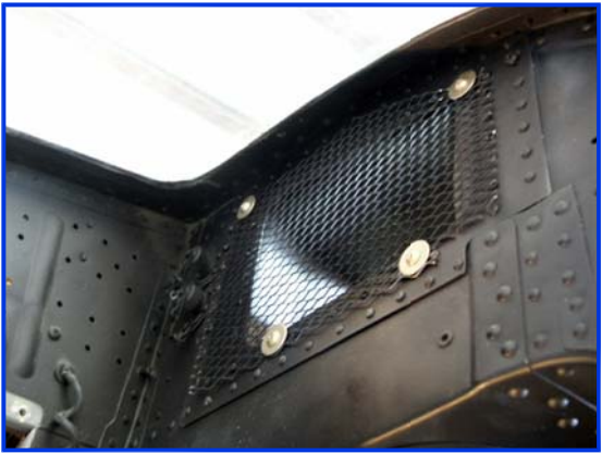
RETURN AIR SCREEN PN: 080036 ABOVE AND BEHIND CO-PILOTS HEAD.
