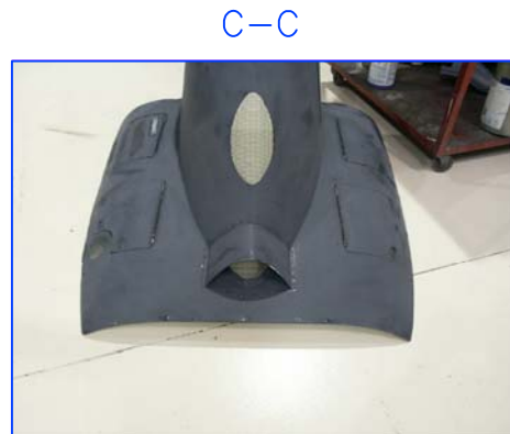
C-C CONDENSER AIR INTAKE IN COWLING, EXISTING
