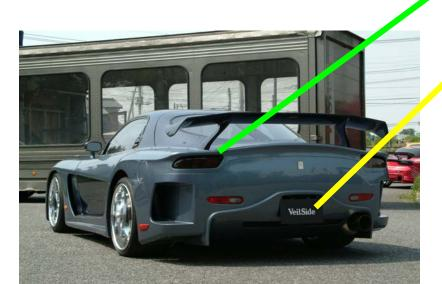
For the isntallation of the tail light assembly, please install bolt from the interior side. Refer to the factory service manual for proper installation, and please make operation check prior to driving.
