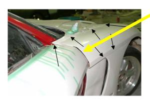
Please proceed to install the front fender, rear fender, and side skirts. Please align all parts together, using spacers where needed so all space between parts are even. Please afix the door panels using epoxy material.
