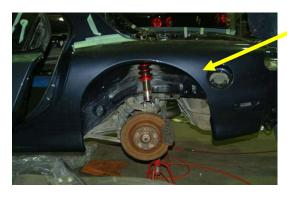
\* The factory rear fenders will be cut to the shape of the VeilSide Fortune model fenders. Please mark and make the cut, welding the inner and outer fenders together.
