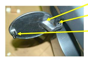
The fuel door will be attached with the supplied steel hinge. The plastic pop-lock mechanism should be installed with self-tapping screws or epoxy.
