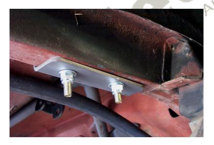
4. Lower the axle and slide the cradle assembly into place. The cradle will be held in place with two 3/8 nylocs and flat washers. Do not tighten these until all the bolts in the cradle have been started.
