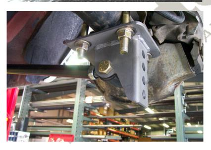
8. The lower axle mount will bolt to the leaf spring pad via the supplied U bolts.
