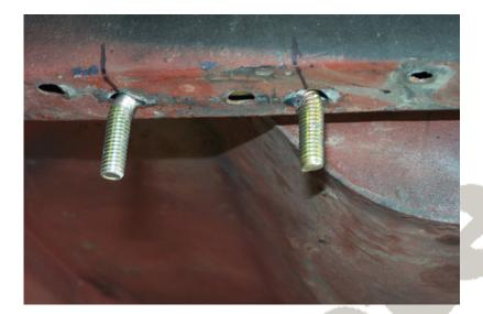
3. The square U-bolts hold the upper cradle in place and will slide through two existing holes. Some cars may not have these holes. In this case use the cradle as a template.
