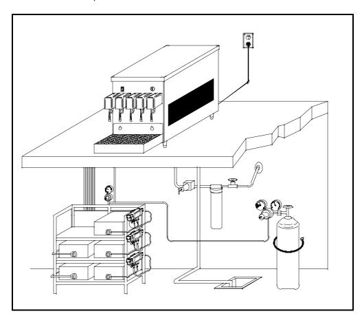
FIGURE 2-1. SAMPLE OF POSSIBLE INSTALLATION.
