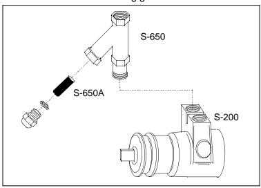
FIGURE 5-1 WATER PUMP, "Y" STRAINER & SCREEN
