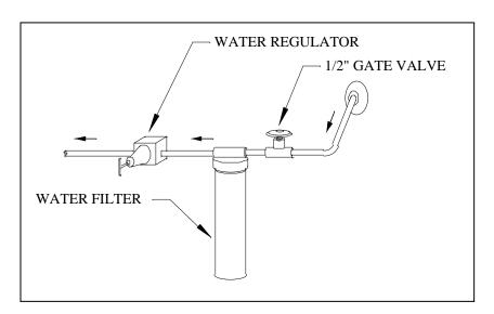
FIGURE 2-4. SUGGESTED WATER FLOW INSTALLATION
