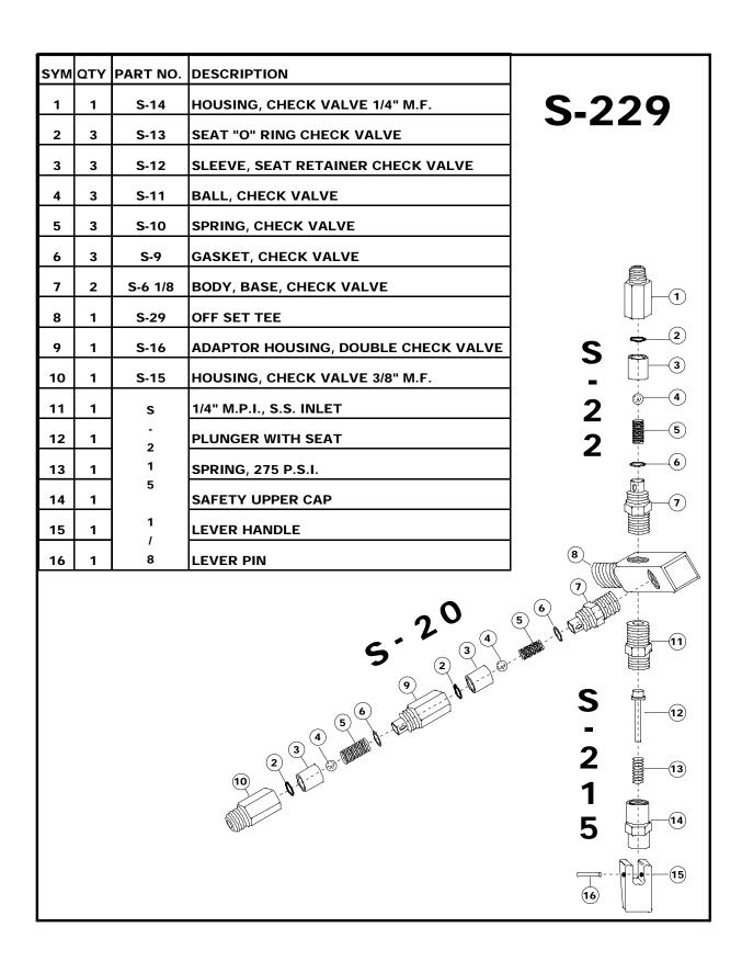
FIGURE 5-3. EXPLODED VIEW CHECK VALVES
