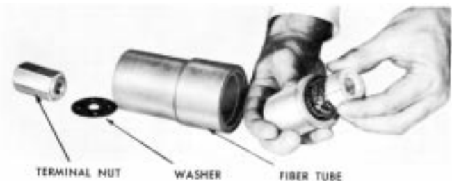
Figure 11 Assembling stationary contact. (Reclosers below serial no. 1001)
