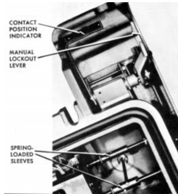
Figure 21 Spring-loaded sleeves of lockout lever and contact position indicator in engaged positions.
