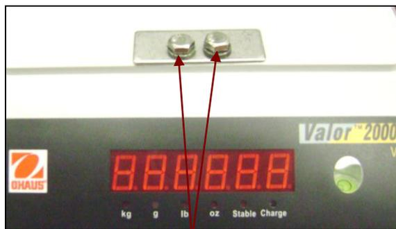
Figure 3-3. Bolts and washers securing Load Cell to Top Housing.
