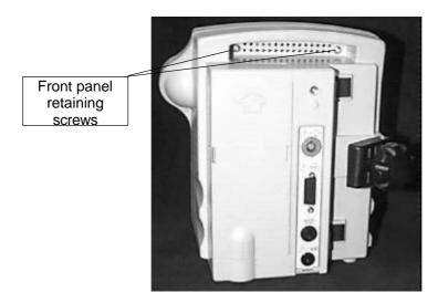
Then carefully pull the top of the front panel away from the rear enclosure. The panel will tilt forwards but is still retained by two plastic clips at its bottom edge. Unhook the front panel from these clips, taking care not to damage them. This is particularly important when refitting the front panel later.
