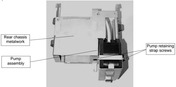
The pump assembly may now be simply removed from the chassis by tilting it forward and pulling.
