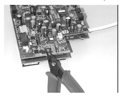
To avoid damage to the p.c.b. interconnection, ensure that the boards are not tilted or twisted relative to each other as they are separated.
