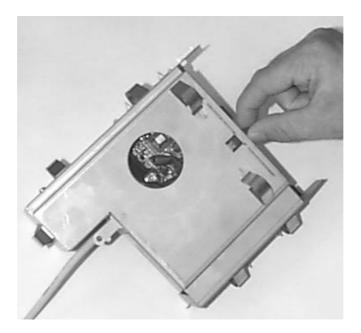
Disconnect pnuematic hose from pump assembly to Main Board secondary pressure transducer on revision 06 units. (Disconnect pressure sensor cable on earlier revisions)
