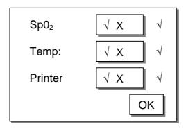
Selection of any of the check boxes causes that monitor feature to be toggled on or off. When on, a tick appears next to the box, denoting that the option is available. Monitors without certain features are supplied without the necessary hardware for that feature and thus will have that option unselected. Selection of **OK** saves changes and returns to the Service menu.
