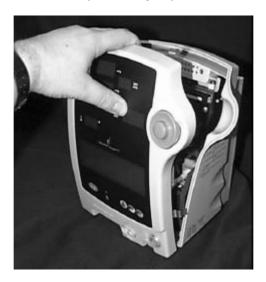
Before the panel can be separated from the case, it is necessary to disconnect the switch board cable, temperature probe cable and  $SpO_2$  sensor cable if fitted.
