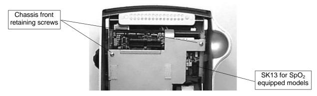
Lift off the front plate complete with SpO<sub>2</sub> module if fitted. This will give access to the top side of the Main Board 8760AB including all the test points and the Flash memory.
