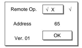
Selection of the **Remote Operation** check box toggles remote operation on and off. When on, a tick appears next to the box, denoting that remote operation (i.e. from the central station) is possible. Selection of the **Address** box allows the monitor's address to be set within the range 1 to 255. Selection of **OK** returns to the Service Menu.
