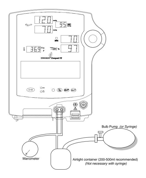
DINAMAP\* COMPACT Calibration check or re-calibration
