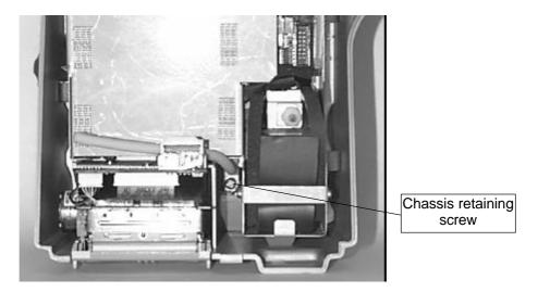
Once the screw has been removed, tilt the chassis forwards and remove the three plugs at the top of the power supply board. From left to right, these plugs connect to the host port, the power input connector and the remote alarm. Disconnect the printer cable from the Printer board 8650AB. The chassis assembly may now be lifted slightly and eased forwards, so that the speaker plug can be removed from the bottom of the power supply board.
