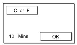
When Celsius is selected, the °C indicator lights. When Fahrenheit is selected, the °F indicator lights. Click on **OK** to clear and save the selection. Note that changing temperature units will clear the trend readings. The user is requested to confirm or cancel this.
