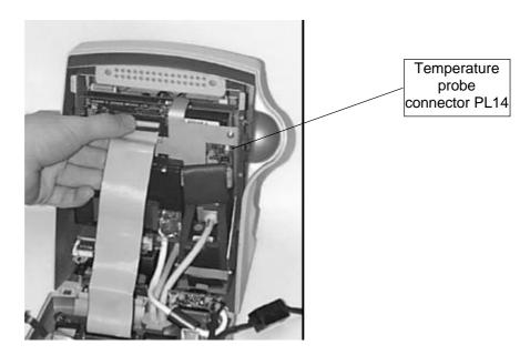
The cable from the Temperature probe socket plugs into connector PL14 on the Main Board and is easily removed.
