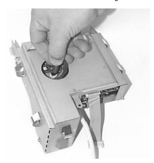
The chassis spade terminal must also be removed. This is located between the top of the chassis and the Power Supply (8620AB) board (Unit revision 04 and 06 only).
