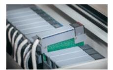
The Programmable Logic Controller (PLC) is easy to trouble shoot and field service. Controller modules simply unplug for immediate replacement.
