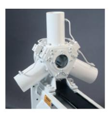
The PQ Tri-lobe rod holder is one of the options available on Series feedframes for the LMA90. Gripping pressure is maintained by high capacity springs acting on three tungsten carbide insert laws.
