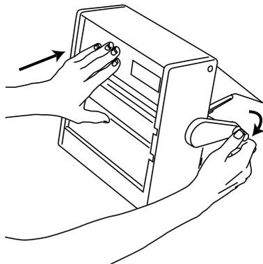
Install feed tray and trim off excess film using cut blade.
