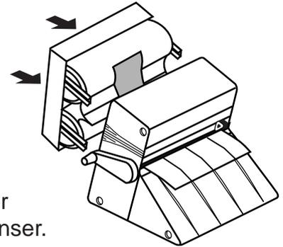
Turn handle clockwise until tool has exited dispenser and film is aligned and wrinkle-free.
