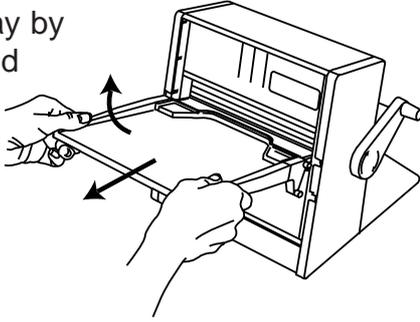
Remove used supply cartridge by pulling outward. If there is film between the rollers, turn handle counter-clockwise.
