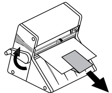
Install feed tray and trim off excess film using cut blade.
