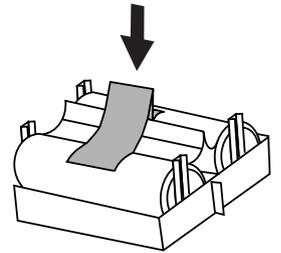
Insert partially used supply cartridge into dispenser. **Note:** tool should be positioned between rubber rollers in dispenser.
