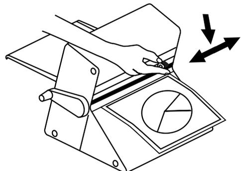
Step 3 - Trim to desired length using the cut blade at the roller exit. Apply pressure down on the orange blade holder and slide to the left or right.
