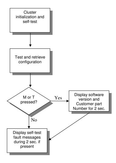
The ignition binary input is used to sense if the key switch is on or off. The system enters start-up mode when the ignition input is active. The system will then go through the functional diagnostic tests described below.
