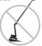
Do not depend on the tilt alarm as a level indicator. The tilt alarm sounds in the platform only when the machine is on a severe slope.
