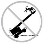
Use extreme care and slow speeds while driving the machine in the stowed position across uneven terrain, debris, unstable or slippery surfaces and near holes and drop-offs. Do not drive the machine on or near uneven terrain, unstable surfaces or other hazardous conditions with the boom raised or extended.
