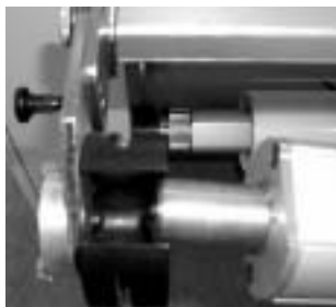
Ball Nose Spring Plunger End
