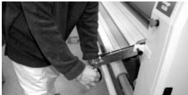
Figure 12. Pivoting Roll Easel Bracket Down
