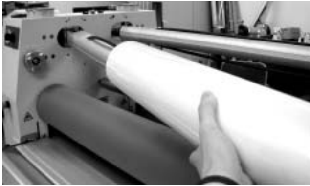
Figure 10. Loading Roll of Material
