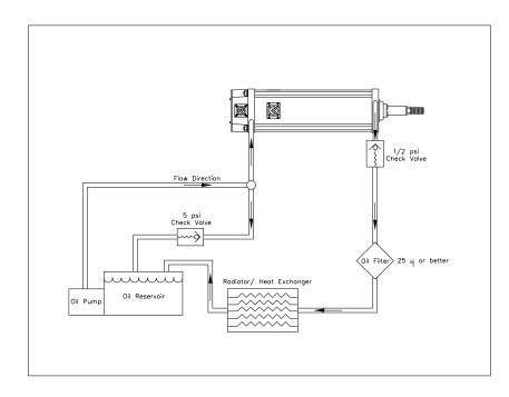
As shown in the schematic to the left, a check valve or other method of pressure regulation should be used to maintain an internal actuator oil pressure of 5 psi.
