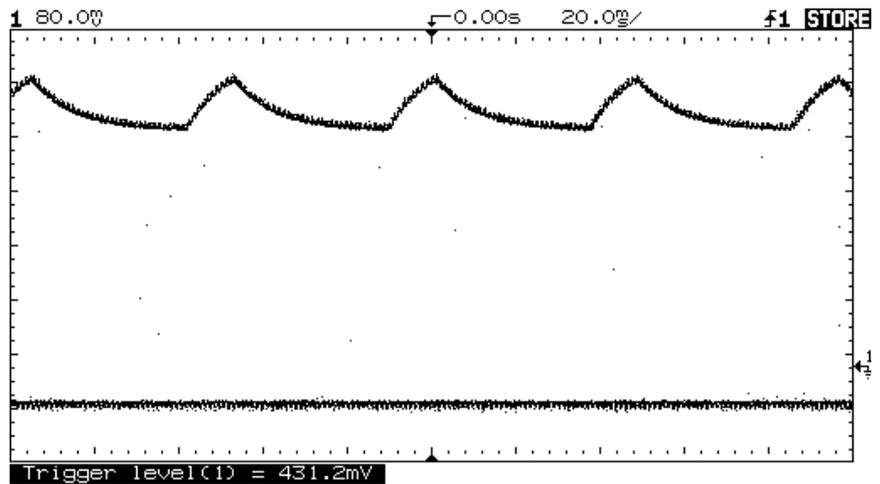
This is a triggered view of the asynchronous noise shown in figure 2-18.
