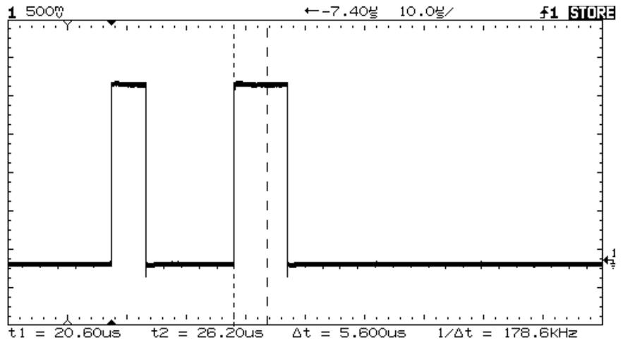
By moving the cursors together, you can check for pulse width variations in a pulse train, as figures 2-15 and 2-16 show.
