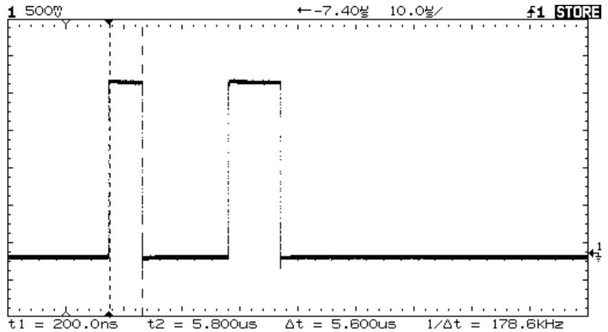
Pressing t1 and t2 softkeys simultaneously causes the cursors to move together when the cursor knob is adjusted.
