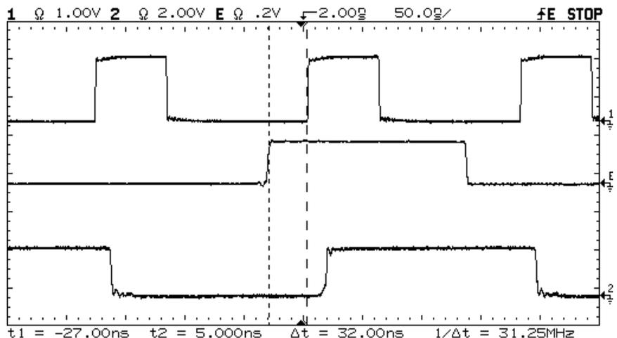
Setup time measurement: channel 1 = clock, channel 2 = Q output, and External Trigger = D input
