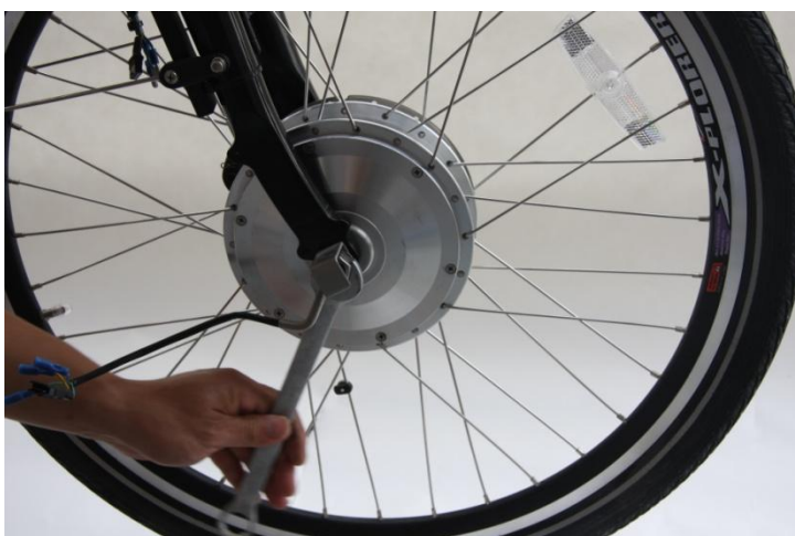
Loosen nut on opposite side using a 19mm or adjustable wrench.
