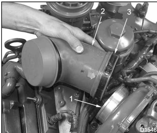
Figure 50 Air inlet duct
