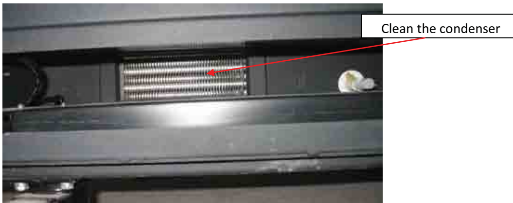
Figure 41 – Clean the condenser
