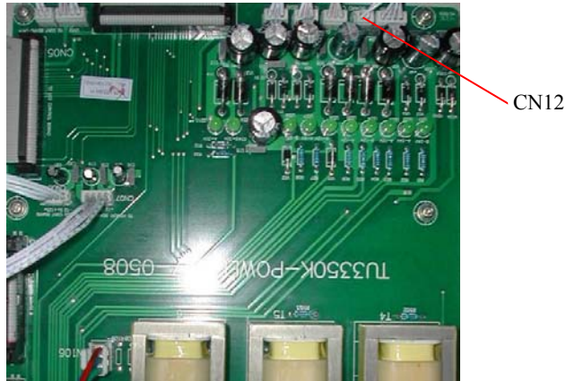
Figure 5-9 Power backup and transfer board CN12
