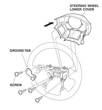
16 Remove the ground tab (one screw).
