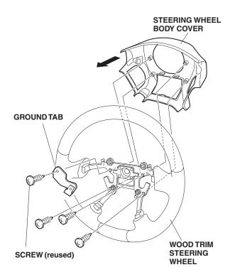
18. Transfer the audio control switch (if equipped) and the cruise control switch to the wood trim steering wheel. Tighten the screws securely.
