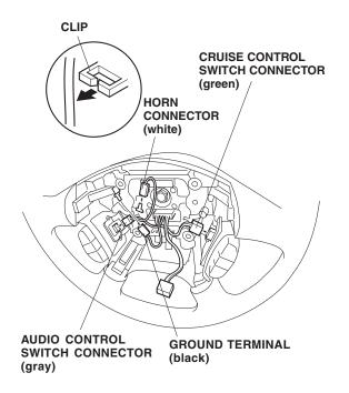
9. Release the airbag harness, the audio control switch harness (if equipped), the cruise control switch harness, and the ground terminal from the four clips on the boss plate cover.
