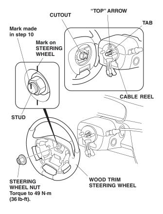
24. Plug in the connectors for the green cruise control switch and the gray audio control switch (if equipped). Connect the black ground terminal to the ground tab, and connect the white horn connector to the horn plate.
