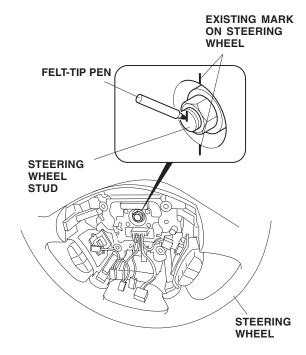
Remove the steering wheel nut. Slowly and carefully remove the steering wheel while routing the wires through the hole in the steering wheel. Be careful not to move the steering wheel during removal.
