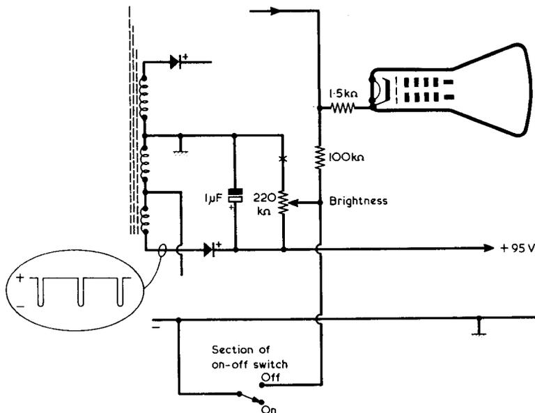
Fig. 7. The higher current 95 volt supply for the video output stage is provided by scan rectification. The cross indicates the position of the open-circuit in the faulty brightness control potentiometer
