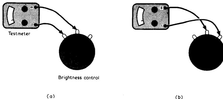
Fig. 1(a). Following Smithy's bidding, Dick checked the continuity of the brightness control potentiometer track in his faulty monochrome TV receiver
