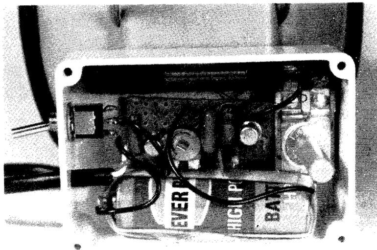
S1 is mounted towards the top of the left hand side panel of the case, and it is important that this be a sub-miniature toggle switch as there is very little space to accommodate it. An entrance hole for the headphone lead is made in the side of the case just below S1.
