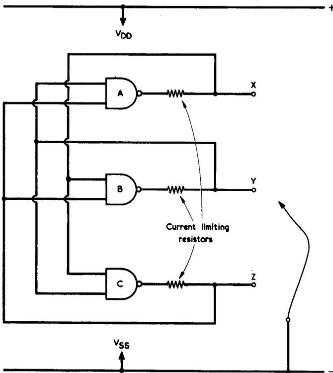
Fig. 2. Adding output current limiting resistors enables the circuit to be changed from one state to another
