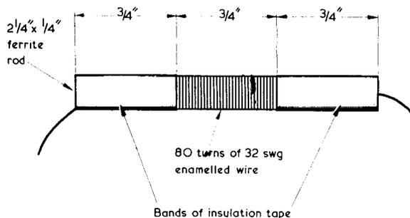
Fig. 2. Details of the ferrite rod aerial winding
