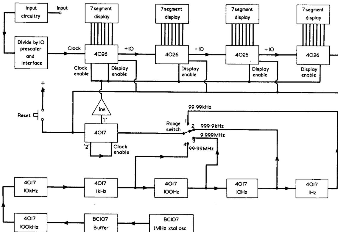
Fig. 2. In practice the frequency meter is more complicated than is evident from Fig. 1. However, the use of integrated circuits simplifies construction to a considerable extent
