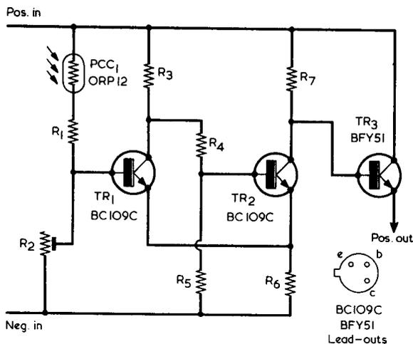
Fig. 2. The auto-dimmer circuit. TR1 and TR2 form a Schmitt trigger which is actuated by the voltage on TR1 base. TR3 is an emitter follower feeding the clock circuit
