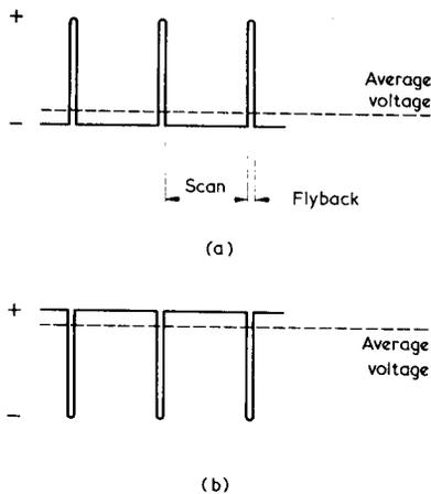
Fig. 5. According to the way connections are made to it, a winding on a line output transformer may produce flyback pulses which are positive-going with respect to chassis, as in (a), or scan pulses which are positive-going, as in (b)
