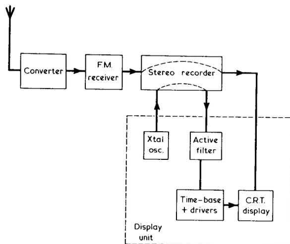
*Block diagram of Satellite Receiving set up*
