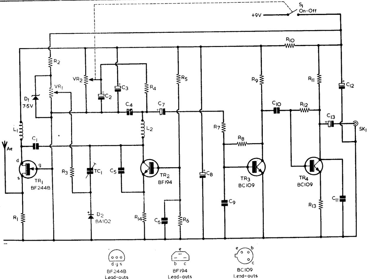
**Fig. 1. The circuit of the single tuned circuit f.m. receiver. Tuning is carried out by VR1 and varicap diode D2**
