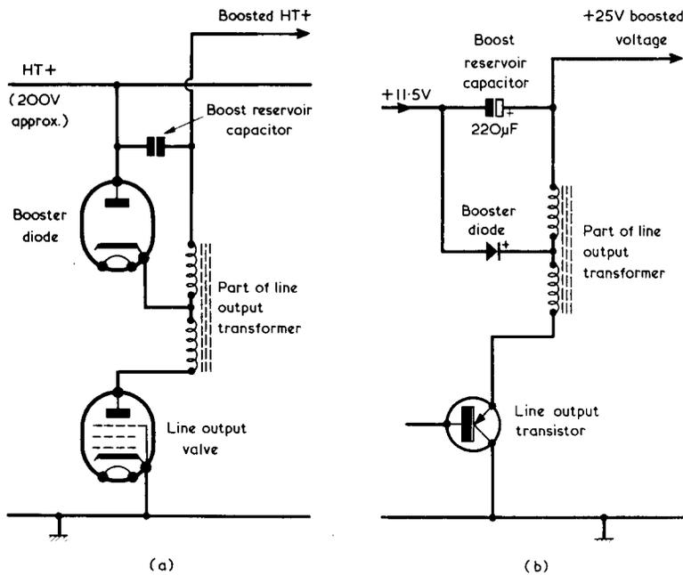
Fig. 3(a). A look at one of the earlier valve line output stages readily demonstrates the formation of a boosted h.t. voltage. With the h.t. voltage shown, the boosted h.t. voltage would be of the order of 500 volts
