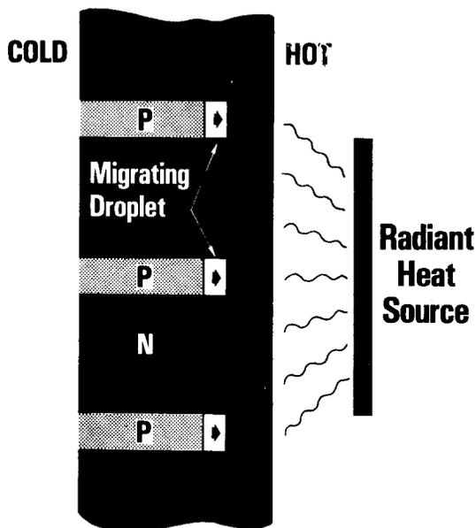
This drawing demonstrates General Electric's "Thermomigration" process. Droplets of dopant in the silicon wafer migrate from the cold side of the slice towards the hot side, taking one-thousandth of the time needed for the introduction of dopants with previous techniques
