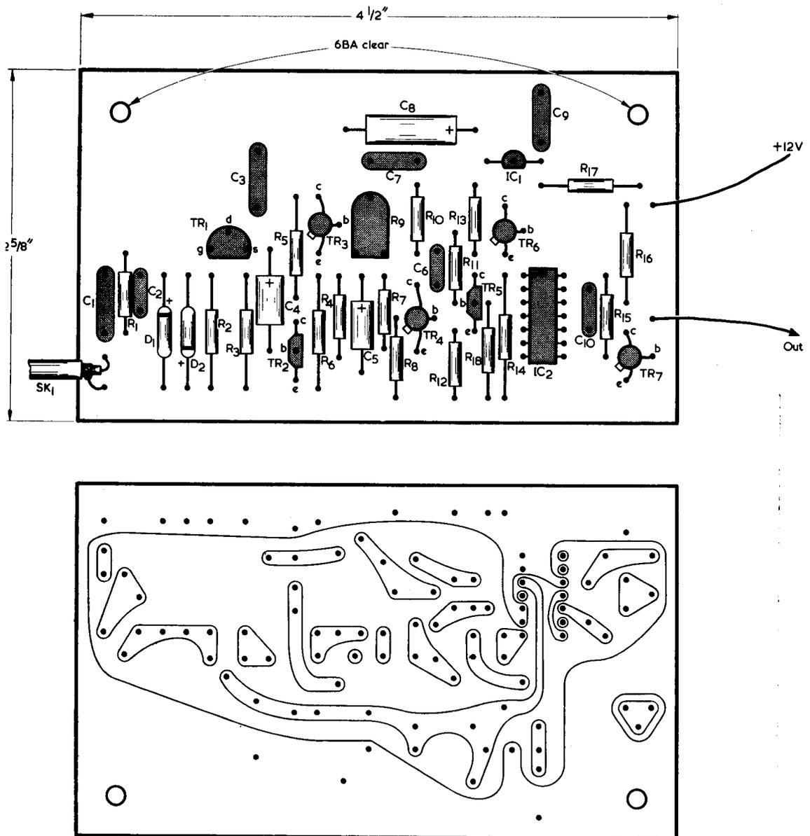
Fig. 4. Component and copper sides of the printed board on which are assembled the input, Schmitt trigger and prescaler stages. The board is reproduced full size
