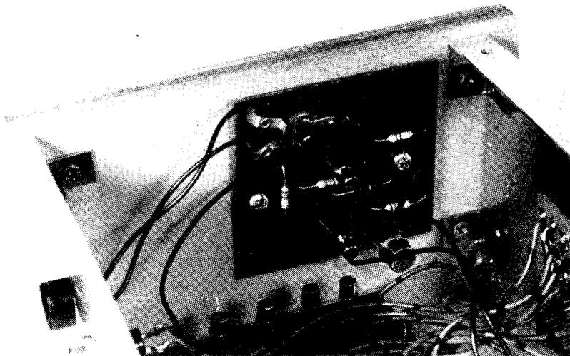
through the track on either side of this break. The hole nearer C1 positive lead-out provides the positive input to the auto-dimmer and the hole nearer C3 takes the auto-dimmer positive output.
