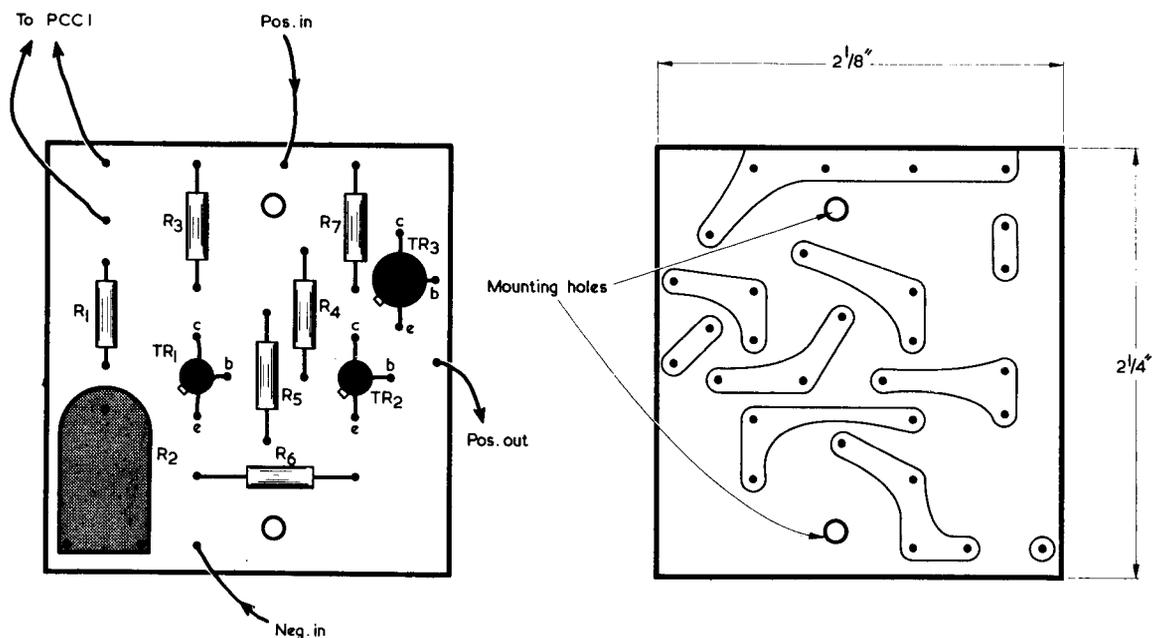
Fig. 3. Details of the printed board, which is reproduced full size
