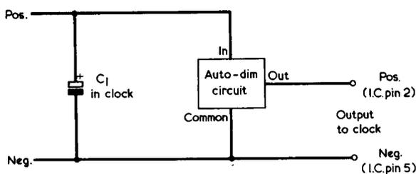
*Fig. 1. How the auto-dimmer unit functions. It takes up the positive and negative outputs of the clock power supply and then varies the positive supply voltage fed to the clock itself*
