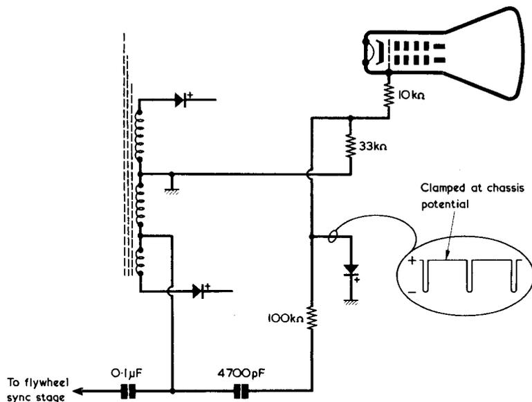
**Fig. 8. Yet some further outputs from the line output transformer. The tap in the lower winding provides line blanking pulses for the picture tube grid together with negative-going flyback pulses to the flywheel sync stage**
