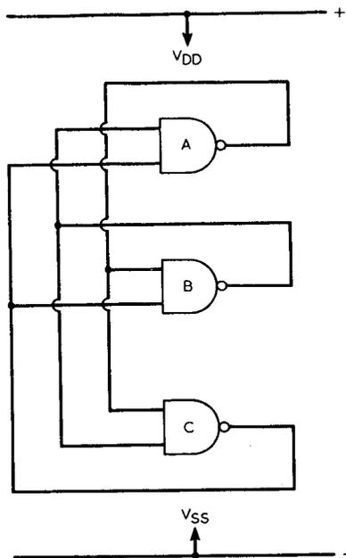
Fig. 1. Theoretical circuit incorporating three CMOS NAND gates. The circuit has three stable states
