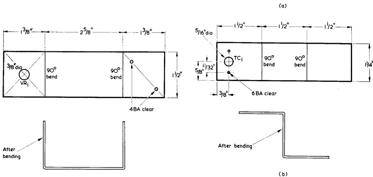
Fig. 3. (a) The mounting bracket for VR1. If this component has a non-standard spindle length, bracket dimensions may need to be modified as described in the text
