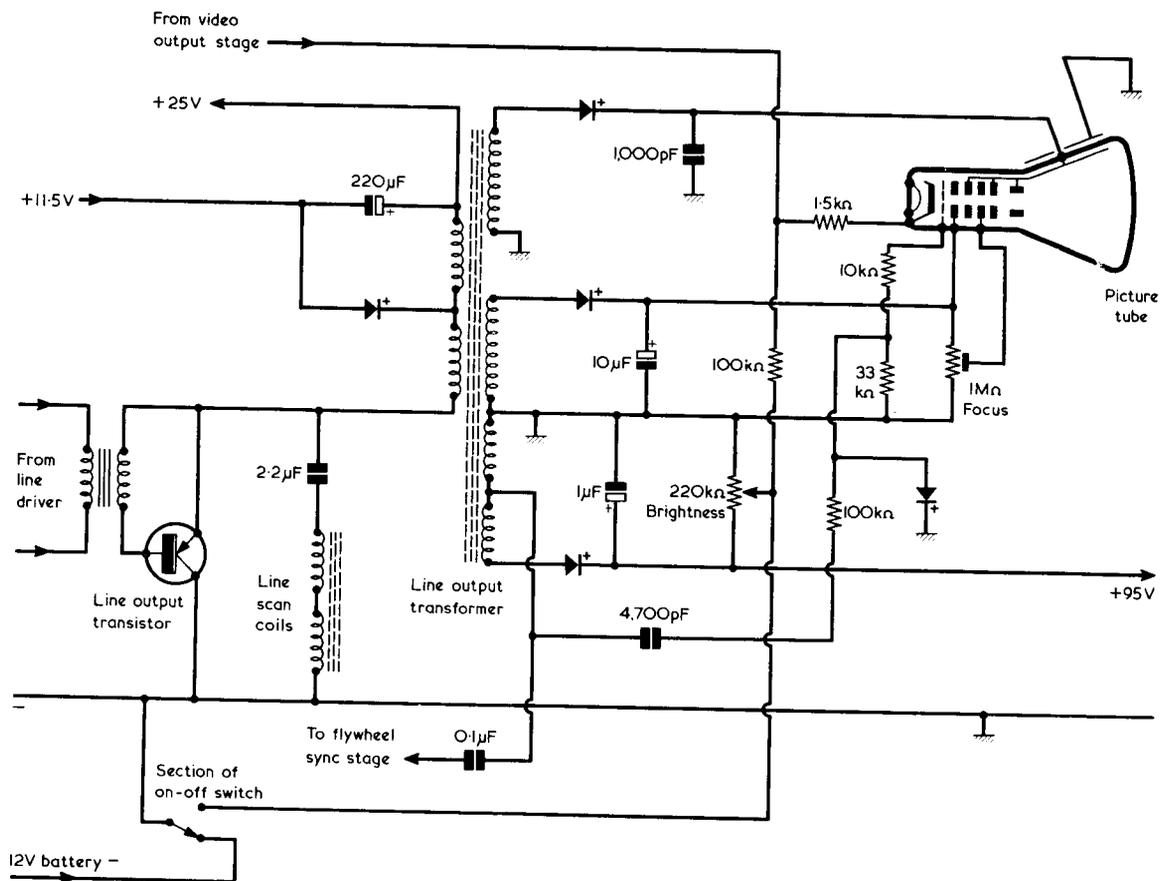
Fig. 2. Line output stage of a monochrome mains/battery television receiver. (This is a slightly simplified version of the circuit employed in the Thorn 1590-1591 Series of television receivers.)
