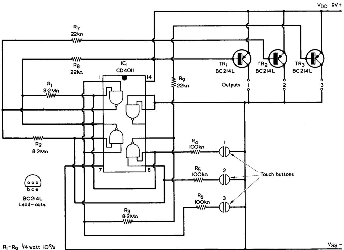
Fig. 3. A practical circuit in which three outputs can be provided by momentarily touching one of the three touch buttons
