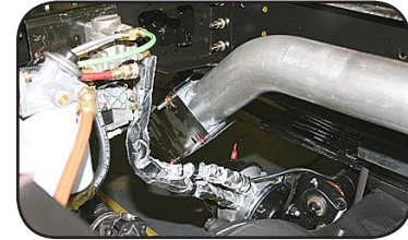
The exhaust systems of 2007 and newer engines incorporate engine-specific Diesel Particulate Filters, which operate at higher temperatures during their Regeneration cycles. The front exhaust pipes are insulated, and heat shields are installed at locations along the exhaust tubing.
