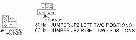
120VAC - JUMPER JP1 TOP TWO POSITIONS 240VAC - JUMPER JP1 BOTTOM TWO POSITIONS
