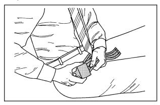
To make the belt longer, tilt the latch plate and pull it along the belt.
