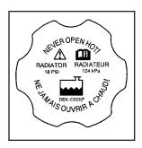
You can remove the pressure cap when the cooling system, including the pressure cap and upper radiator hose is no longer hot. Turn the pressure cap slowly counterclockwise.
