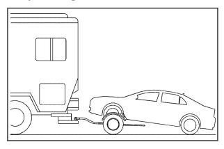
The vehicle can be towed with its front wheels on a dolly. To tow the vehicle using a dolly:
