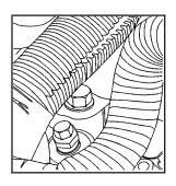
Open the coolant air bleed valve located on the thermostat housing, near the upper radiator hose.
