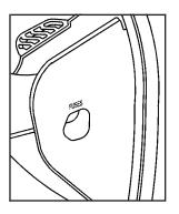
The instrument panel fuse block is located on the passenger side of the instrument panel. Pull off the cover labeled FUSES to expose the fuse block.
