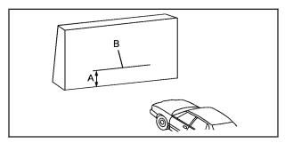
3. At the wall measure from the ground upward (A) to the recorded distance from Step 3 and mark it.
