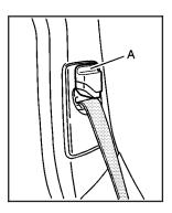
Press down on the release lever (A) and move the height adjuster to the desired position.
