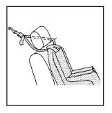
If the position you are using has a fixed headrest or head restraint and you are using a dual tether, route the tether around the headrest or head restraint.
