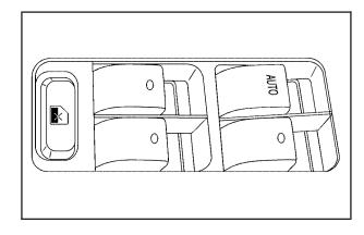
The switches on the driver's door armrest are used to control each of the windows. The power window switches work while the ignition is in ON/RUN, ACC/ACCESSORY, or while Retained Accessory Power (RAP) is active. See *Retained Accessory Power (RAP)* on page 2-22. Each passenger door has its own window switch.
