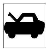
Pull the interior hood release handle with this symbol on it. It is located to the left of the steering column below the instrument panel.
