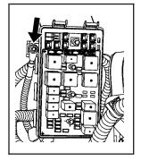
If your vehicle has a V6 engine, to uncover the remote positive (+) terminal, press the tab at the bottom of the fuse block and lift the cover up.
