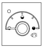
The fuel gage indicates about how much fuel is left in the fuel tank when the ignition is on. When the indicator nears empty, there is still a little fuel left, but you should get more fuel soon.
