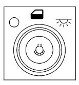
The interior lamps control is located next to the exterior lamps control and to the left of the steering wheel on the instrument panel.
