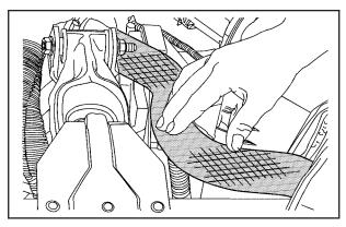
Start the engine and let it run until you can feel the upper radiator hose getting hot. Watch out for the engine cooling fans.
