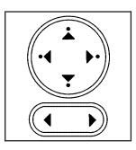
Controls for the outside power mirrors are located on the driver's door armrest.
