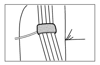
Be sure that the belt is not twisted and it lies flat. The elastic cord must be under the belt and the guide on top.
