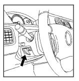
The lever used to tilt the steering wheel is located on the left side of the steering column.
