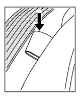
To lower the rear seatback, pull the tab located on the outboard side of the seatback and fold the seatback forward.
