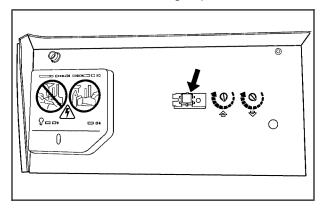
After Steps 1 through 6 have been completed, locate inside the garage the garage door opener receiver (motor-head unit). Locate the "Learn" or "Smart" button. The name and color of the button may vary by manufacturer.
