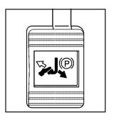
To set the parking brake, hold the regular brake pedal down, then push down the parking brake pedal.
