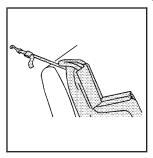
If the position you are using does not have a headrest or head restraint and you are using a single tether, route the tether over the seatback.
