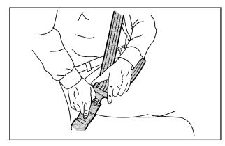
To unlatch the belt, just push the button on the buckle. The belt should return to its stowed position. Slide the latch plate up the safety belt webbing when the safety belt is not in use. The latch plate should rest on the stitching on the safety belt, near the guide loop on the side wall.
