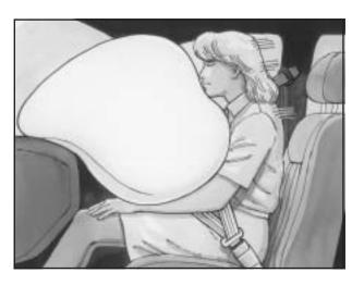
The right front passenger airbag is in the instrument panel on the passenger side.
