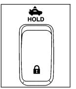
Press and hold the top of the driver's or front passenger's power door lock switch to unlock the trunk.
