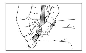
3. Push the latch plate into the buckle until it clicks. If you find that the latch plate will not go fully into the buckle, check if the correct buckle is being used. Pull up on the latch plate to make sure it is secure.
