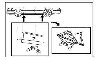
Find the jacking location using the diagram above and corresponding triangular-shaped hoisting notches located on the underside of the vehicle's plastic molding.
