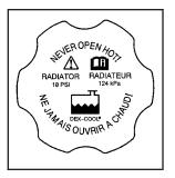
You can remove the radiator pressure cap when the cooling system, including the radiator pressure cap and upper radiator hose, is no longer hot.
