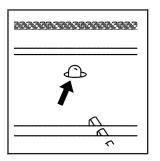
Your vehicle may have a red light located on top of the instrument panel, toward the center of the vehicle and near the windshield, that will flash slowly when the system is armed.
