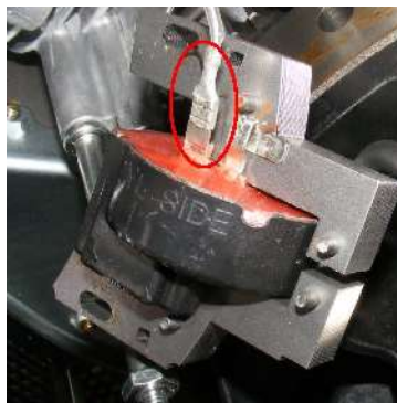
"Kill" terminal connection
