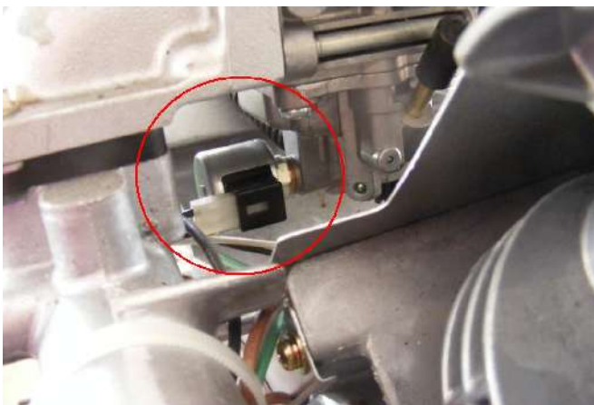
Vanguard engine anti-afterfire solenoid
