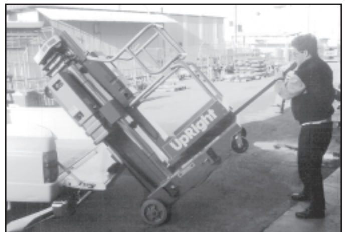
Figure 7: Tilting machine onto or off of a vehicle
