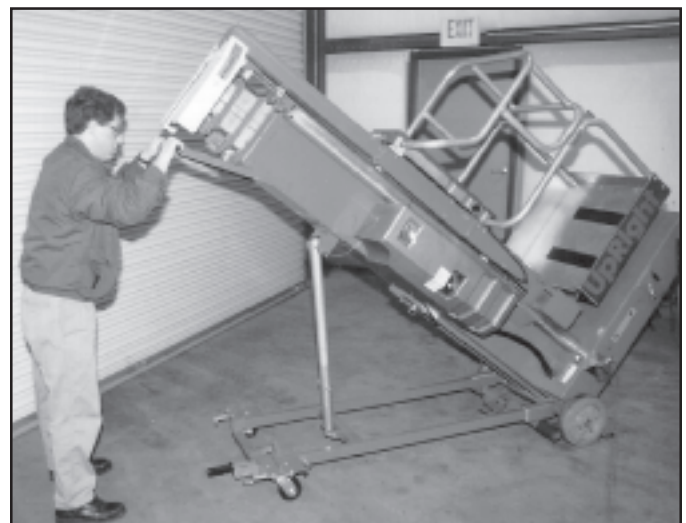
Figure 10: Compressing cylinder assembly
