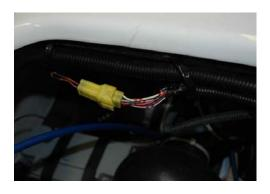
Remove the dust cap from the diagnostic connector, attach the STX-100 Di Main Diagnostic cable to the yellow diagnostic connector on the ski.
