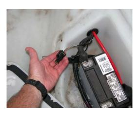
Remove the dust cap from the connector, and attach the Main Diagnostic cable to the diagnostic connector. NOTE: On 2007-2009 models, the Main cable connects directly to the connector on the ski. On 2010 models, you must first attach the 2010+ Adapter cable to the Main cable, then connect the 2010+ Adapter cable to the diagnostic connector on the ski.
