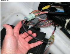
Once the Immobilizer Bypass cable is installed, connect he two small white one-pin connectors together on this cable:
