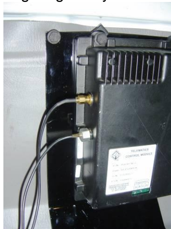
Figure 32 - Antenna cables connected to module
