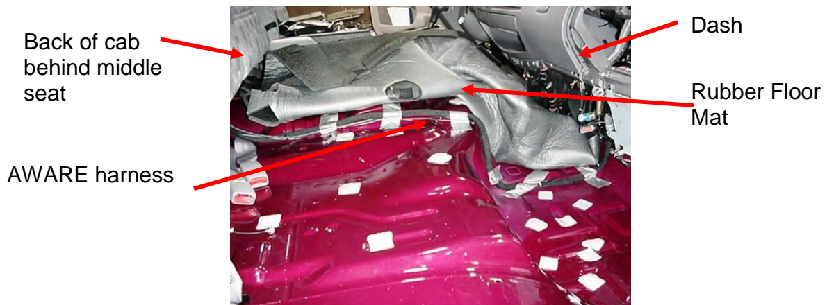
Figure 14 –AWARE Harness along floor under rubber mat
