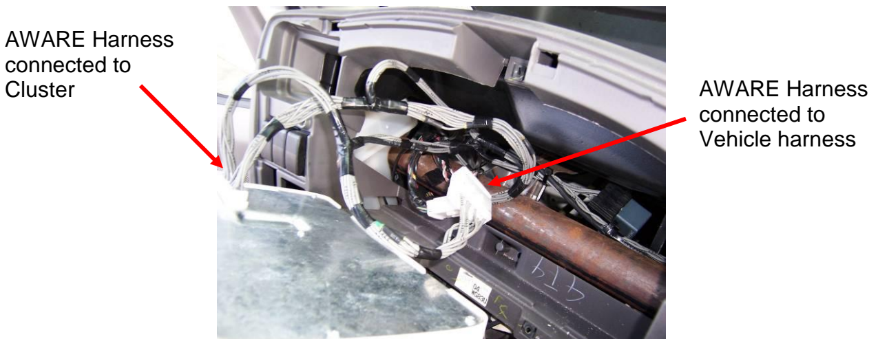
Figure 17 –Harness connection to vehicle harness & instrument cluster
