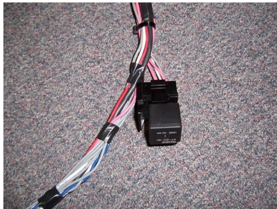
Figure 38 – Relay inserted into harness connector
