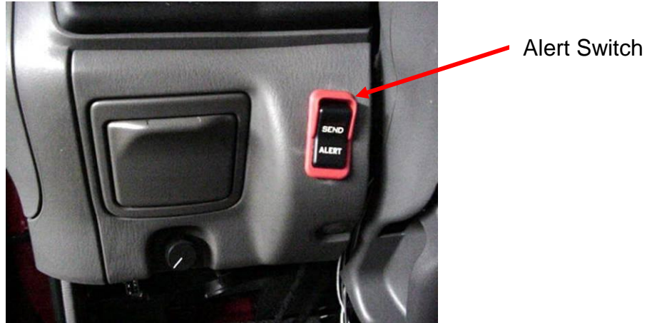
Figure 34 - Driver Alert Switch Installed
