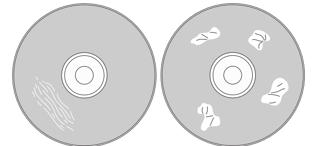
Wrinkle in film caused by excessive heat
