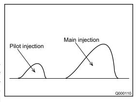
injected before ignition increases, resulting in explosive combustion together with ignition, and an increase in the amount of NOx and noise. Therefore, by providing a pilot injection, the initial injection rate is kept to the minimum required level dampening, the explosive first-period combustion and reducing NOx emissions.
