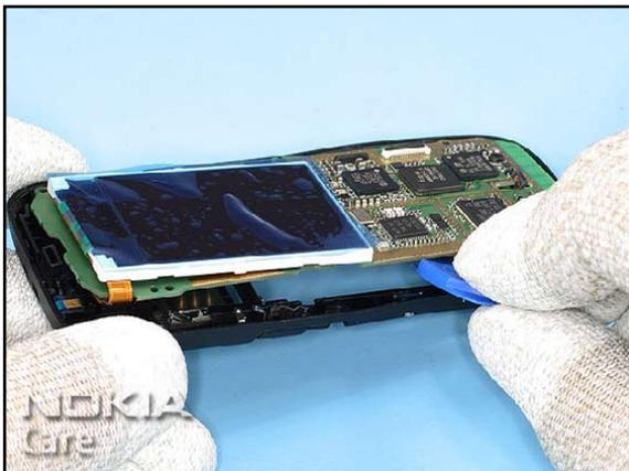
18. Unlock the clips of the D-COVER with the SRT-6...
