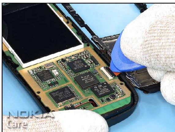
12. Be double careful while opening the connector with the SRT-6.
