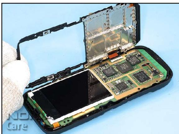
11. Carefully flip over the C-COVER ASSY now, keep in mind that the flex foil is still connected.
