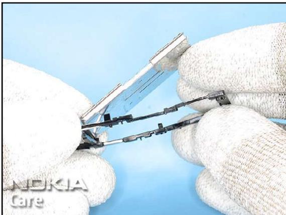
16. Separate the ENGINE SHIELDING ASSY from the C-COVER.
