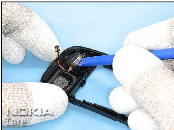
24. Careful lever out the glued in VIBRA MOTOR.
