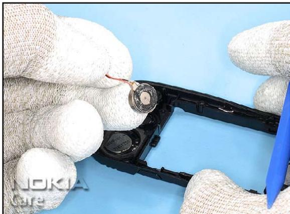
25. The adhesive gasket should stay at the VIBRA MOTOR. Mind that no adhesive residues remains in the cover before replacing a new VIBRA MOTOR. The disassembling procedure is now completed.
