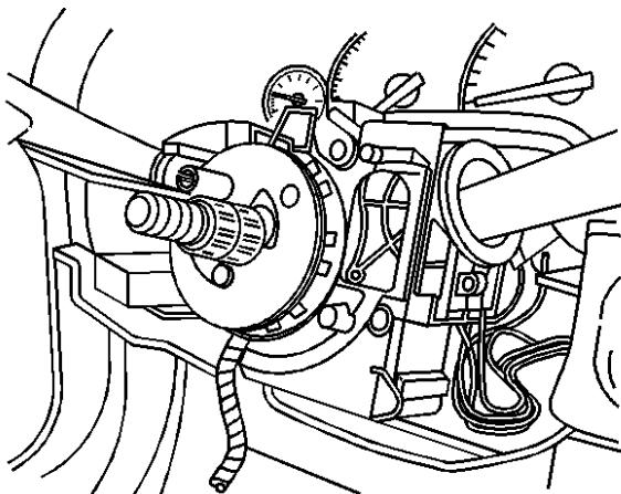
13. Disconnect the ECL electrical harness (located on the right lower side of the steering column) to the I/P main harness.
