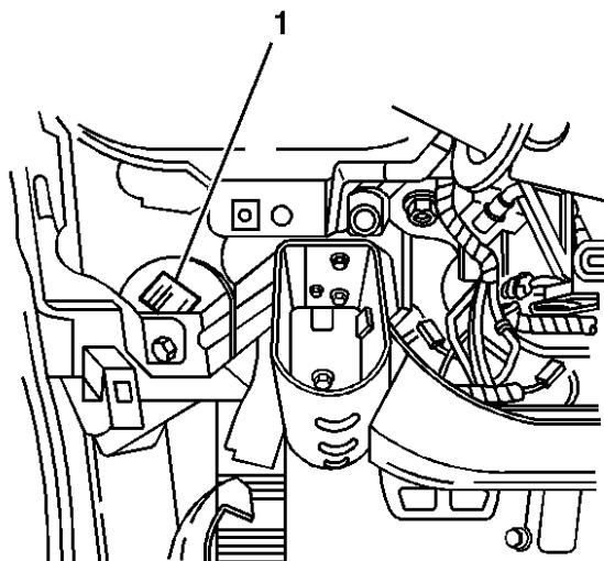
16. Route the new jumper wire and relay harness over the knee bolster (styrofoam and metal construction). The new relay (1) must be mounted to the left I/P brace with a zip tie as shown.
