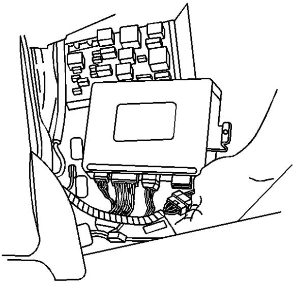
3. Disconnect the green 16-way connector from the BCM. The proper connector is illustrated. (BCM rotated 90 degrees)
