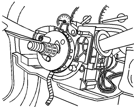
12. Remove and discard the Steering Column Lock/Cam Orientation plate using the J 38364.
