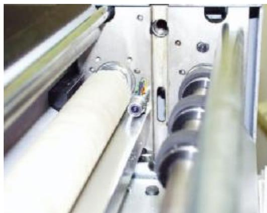
The **Lead Edge Sensor** registers the lead edge of the sheet to within 0.1 mm. Its correct setting is extremely critical to the performance of the machine and **any adjustment of its sensitivity will require re-calibration of the machine.**
