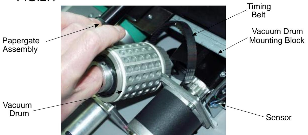
**VACUUM DRUM FEED BELT REMOVAL / REPLACEMENT.**
